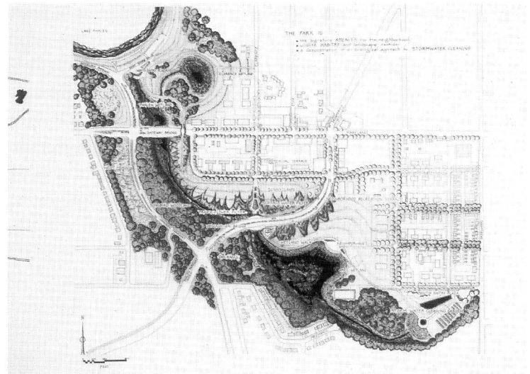
Figure 5. The design for the Phalen Wetland Park as it is envisioned for the current site of the shopping center includes a woodland corridor, filter strips of native prairie and wet meadow plants, and a storm-water cleaning garden.
