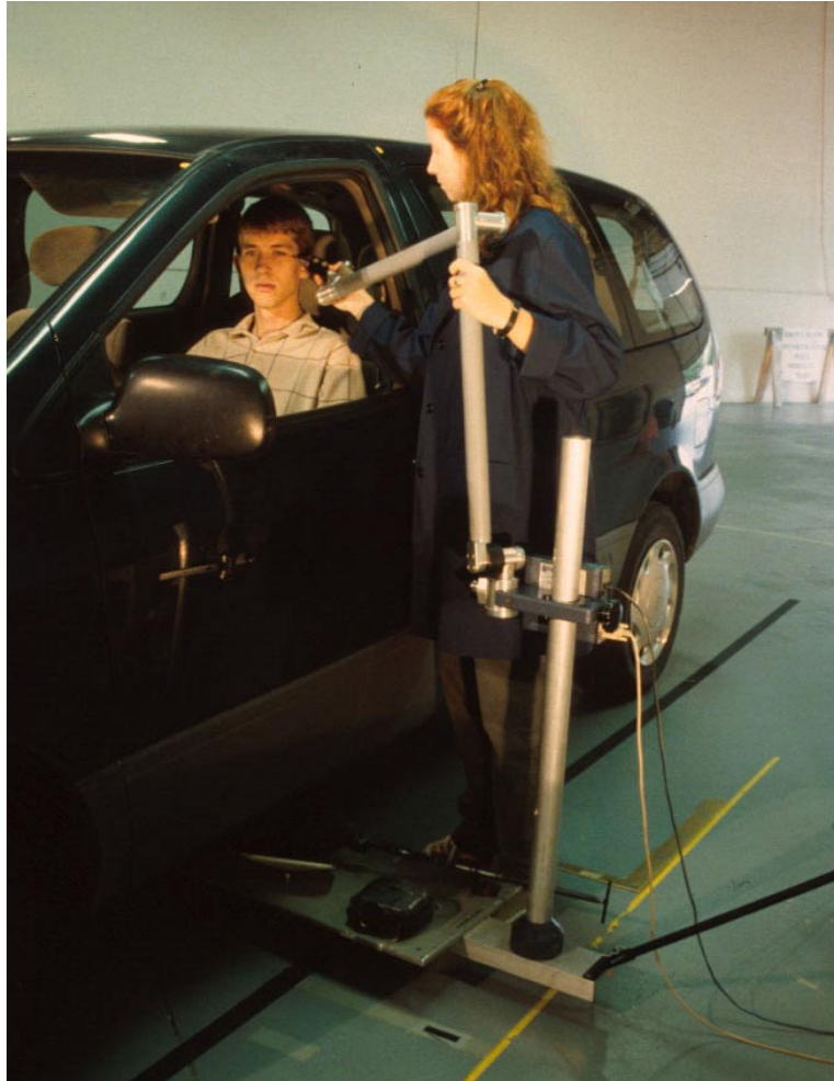
Figure 3. FARO Arm coordinate measurement machine used to record vehicle geometry and driver eye locations.
