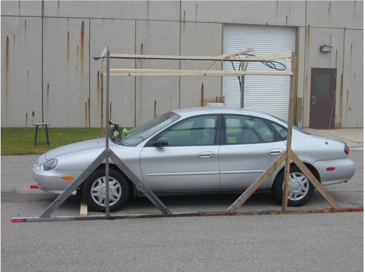
Figure 5. Rigging supporting the overhead sprinkler system used to simulate rain.
