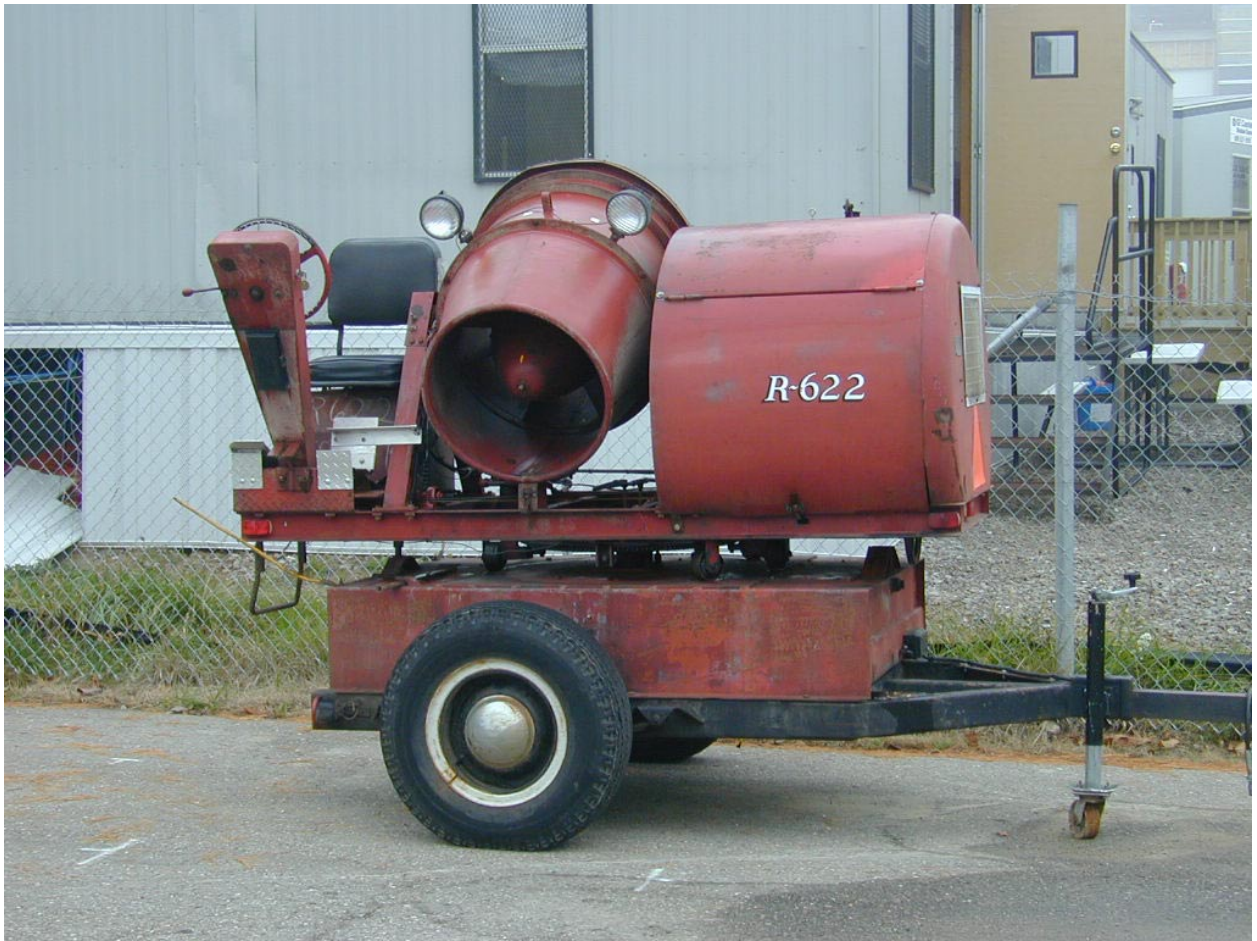
Figure 4. The rotary-turbine wind machine used to simulate air moving over a vehicle in motion.
