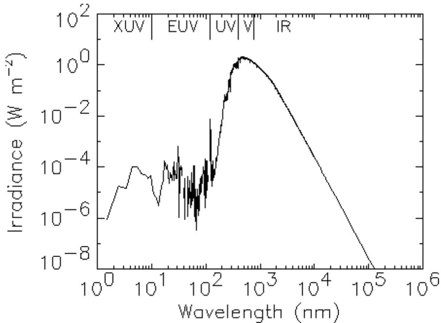
Figure 4. The solar spectrum from 1 to 1,000,000 nm (Tobiska et al., 2000).
