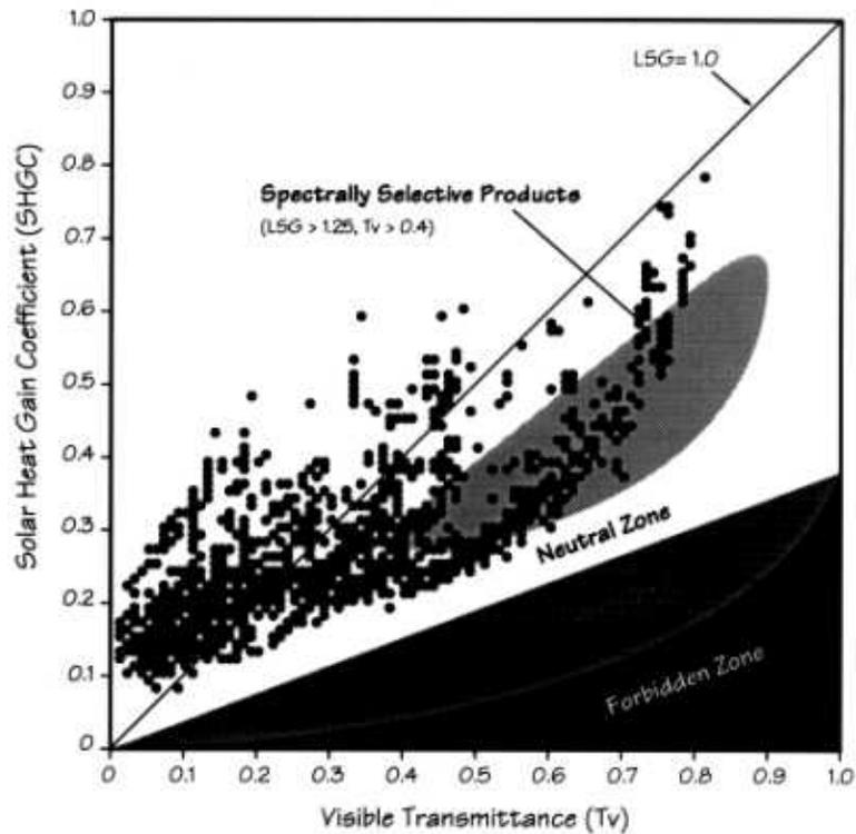
Figure 5. Center-of-glass properties of commercially available, dual-pane, spectrally selective glazing, coatings, and films for commercial applications (Lee, 1998).
