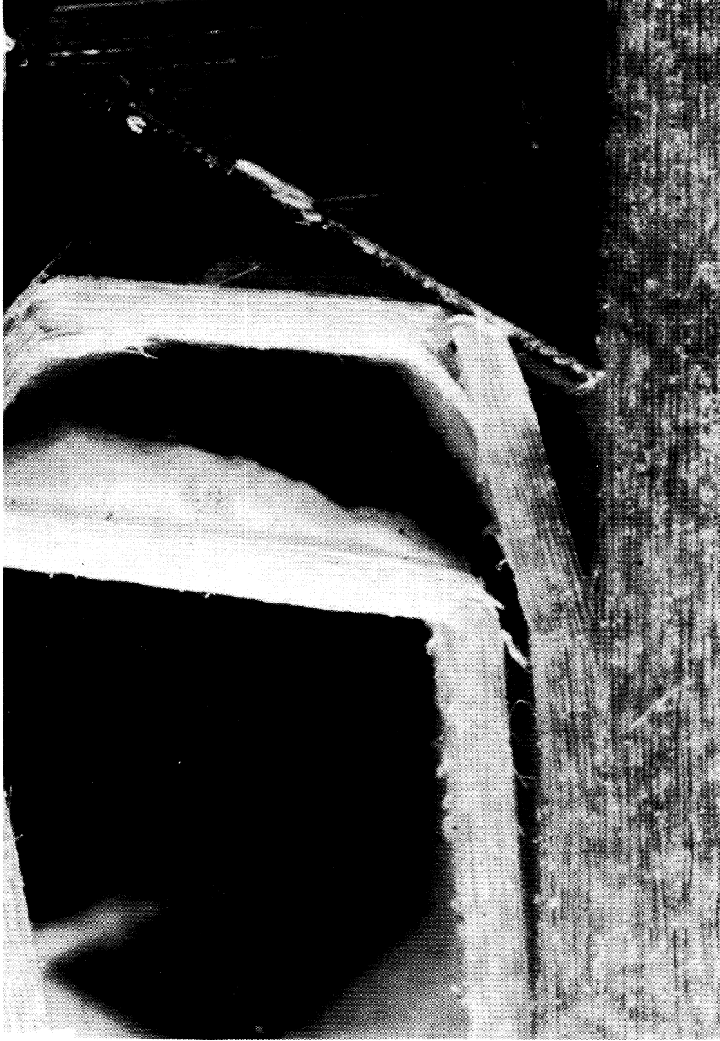
Fig. 21. -- The Type I chip, showing splitting ahead of the tool edge and failure of chip as a cantilever beam.
