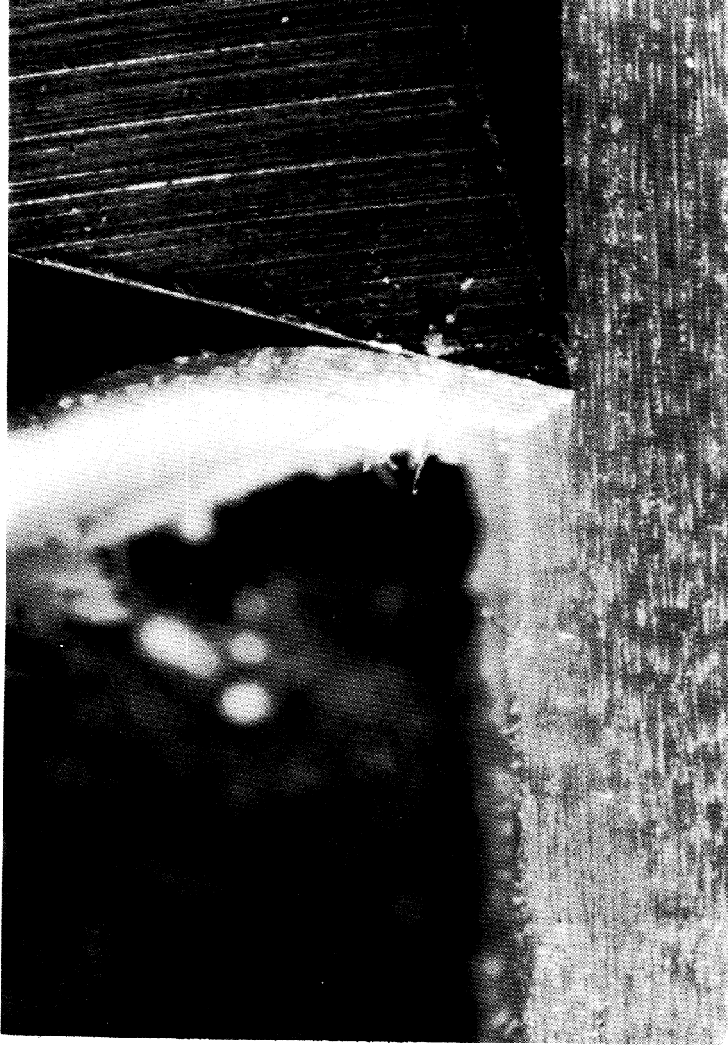
Fig. 22. - - The Type II chip, showing wood failure along a plane extending from the tool edge to the work surface.
