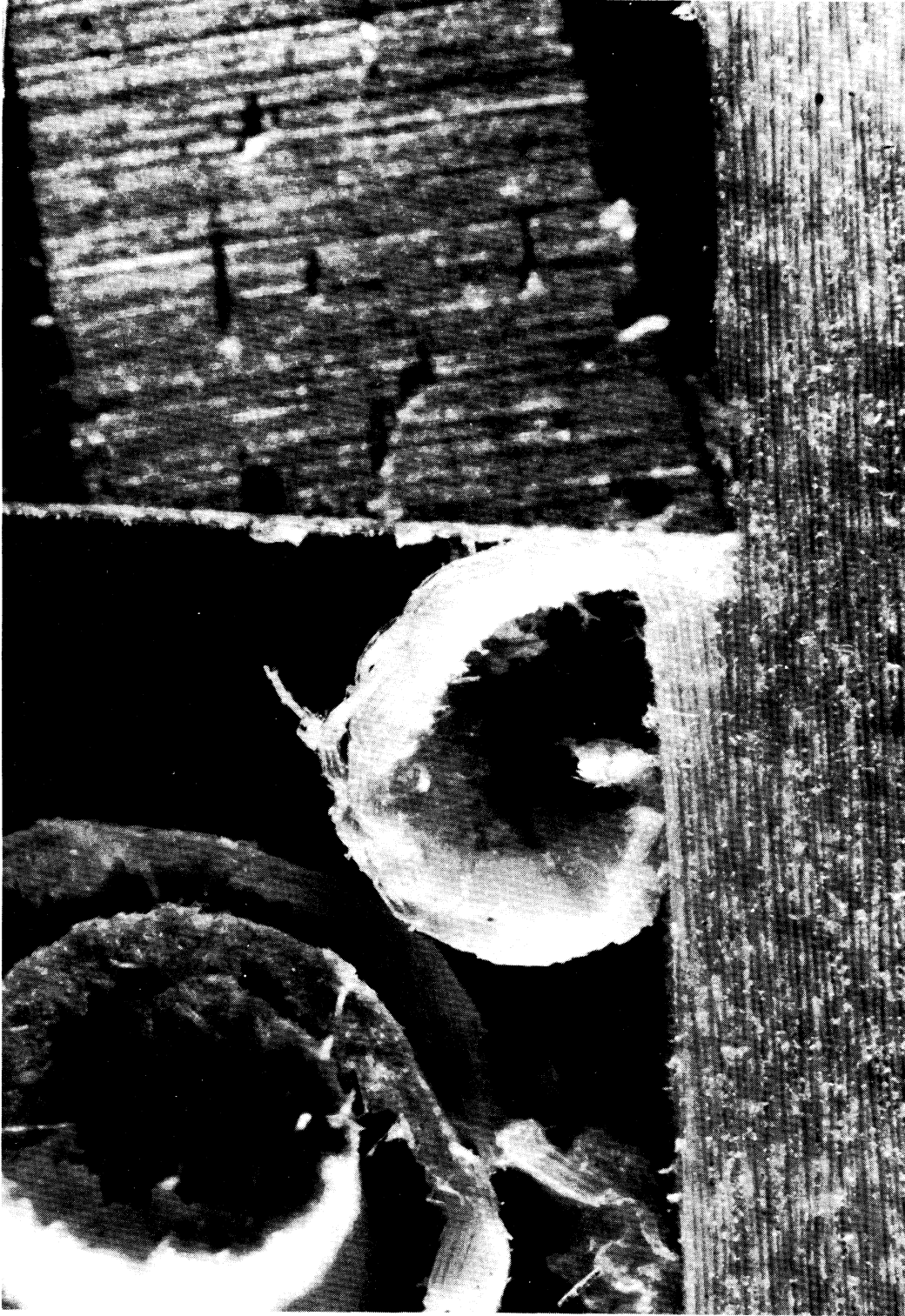
Fig. 34. - - The Type III chip with built-up edge of compacted wood.
