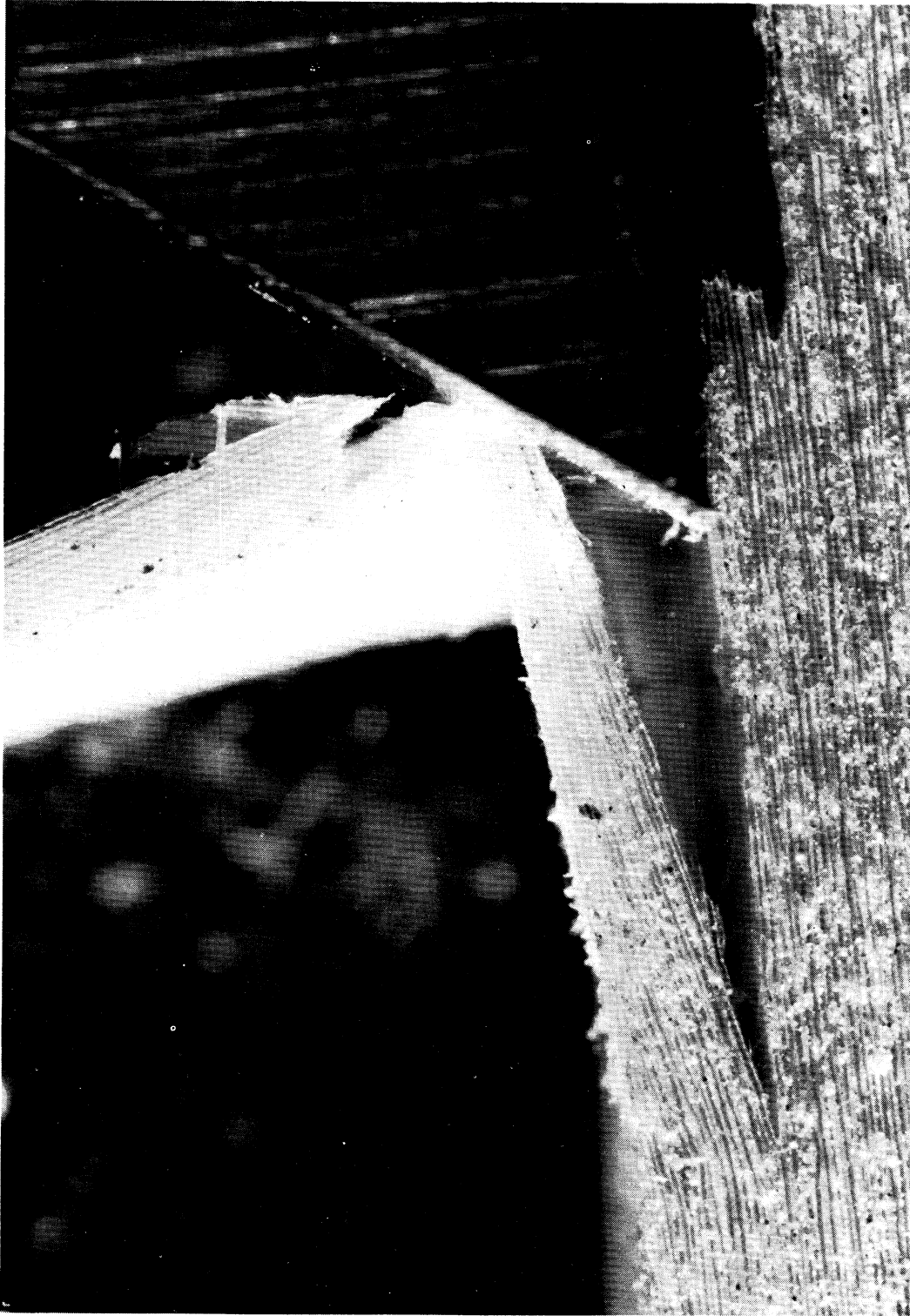
Fig. 28. --Formation of the Type I chip when cutting against wood grain making 5-degree angle with the tool path.
