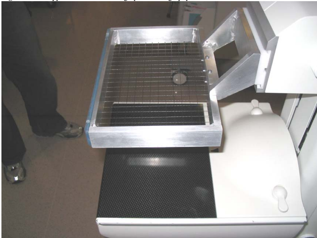
Figure 6: Prototype fitted into the Senograph mammography machine
