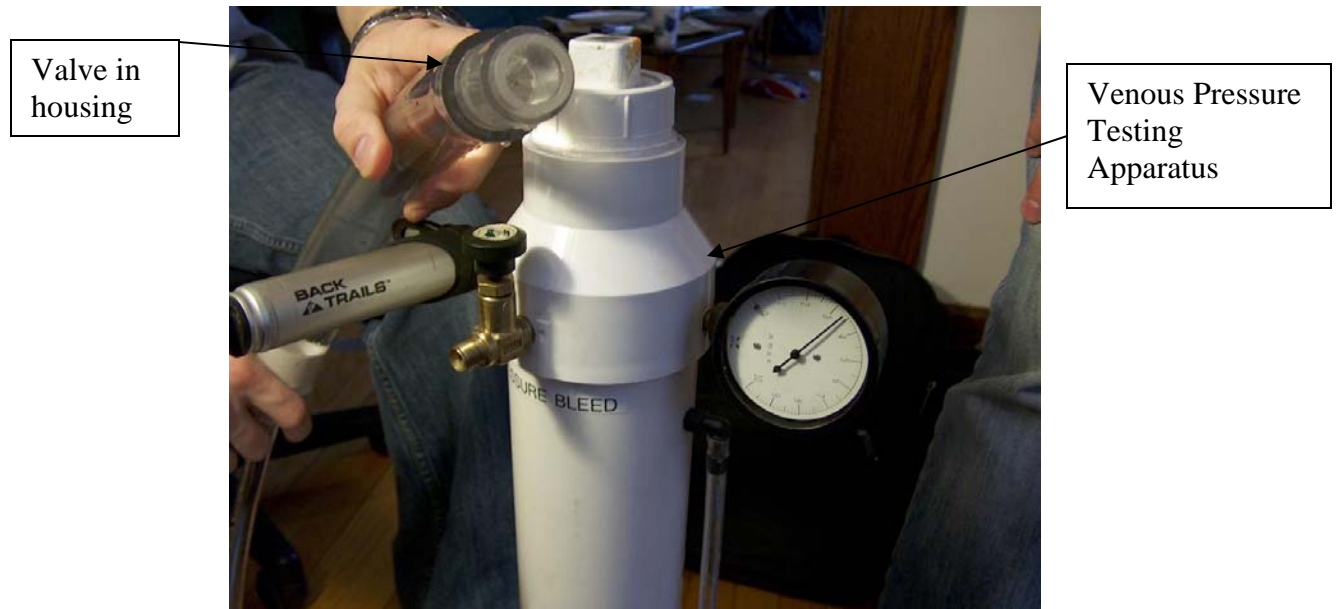
Figure 38: Leak testing setup
