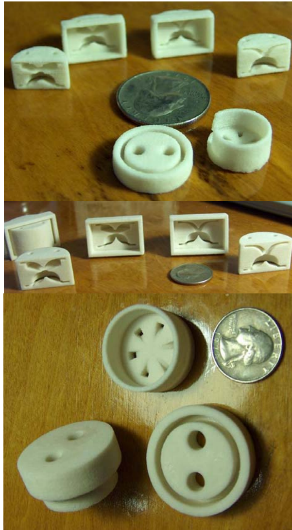
Figure 34: Iterations of prototype molds, Top 1 st Generation, Bottom 2 nd Generation
