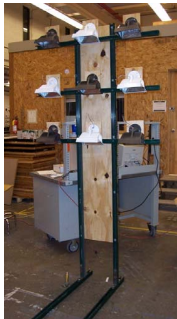
Figure 8: Artificial light source constructed for SHGC testing
