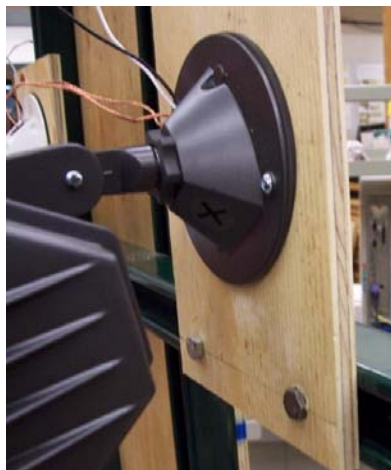
Figure 10: Lights were mounted to the Uni-Strut cross-sections using wood planks and bolts
