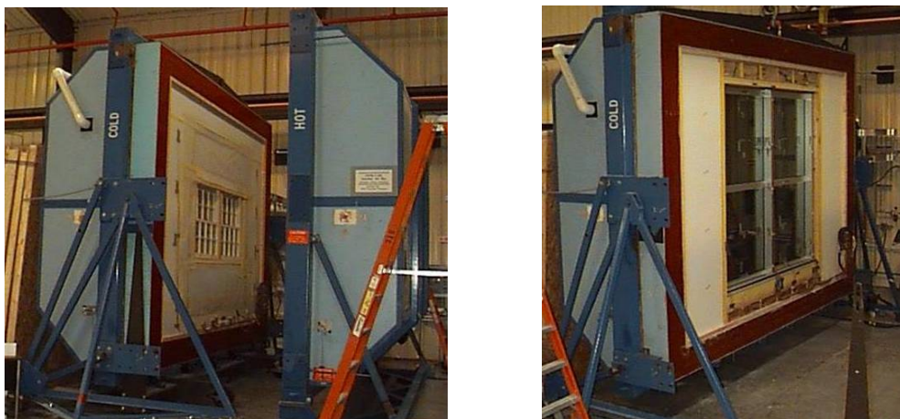
Figure 7: Rotatable guarded hot box [12]
