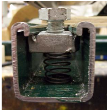
Figure 9: Uni-Strut nuts and bolts used to construct the artificial light source
