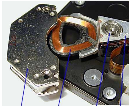
Figure 11: Voice coil concept. A rotary voice coil motor could be placed underneath each button.
