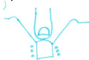
Figure 13: Speaker motor concept. This concept directly uses the motor as a button.
