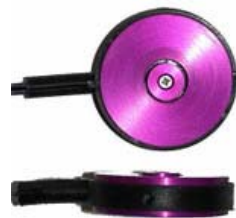
Figure 16: Electromagnetic and pneumatic tactors. Tactors produce a tapping sensation in the finger through vibrations (electromagnetic) or air pulses (pneumatic) [14, 15].
