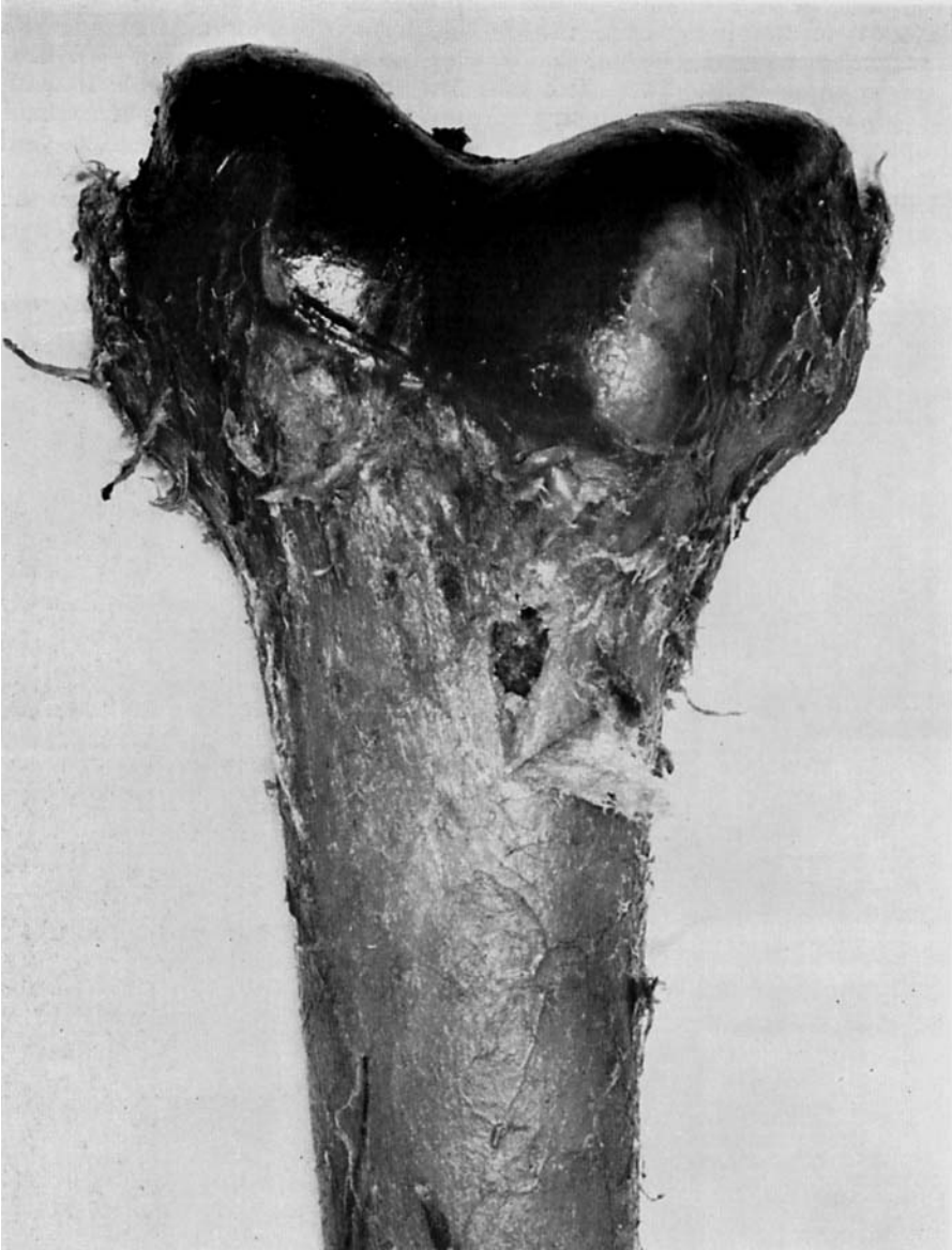
Fig. 3 Exit hole of an embalmed human femur impacted by a one-fourth inch steel sphere at 700 ft/sec.
