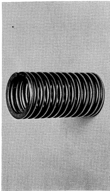
Fig. 61. Bimetal system composed of Inconel X thin-walled tubing 0.09375 in. ID, 0.119 in. OD with core 40% nickel-balance iron alloy 0.09375 in. diameter. Outside diameter 1.0 in., n = 9-1/2 . View before test.
