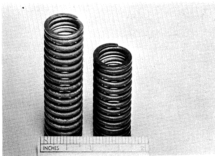
Fig. 6. 40% nickel alloy coils. Wire diameter 3/32 in., c = 7.0 , n = 15 , p = 9/64 in. (on left); wire diameter 3/32 in., c = 6.95 , n = 10 , p = 9/64 in. (on right).
