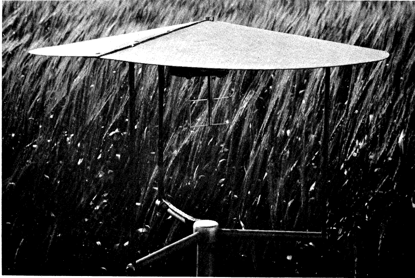
Figure A.8(a). Roto-bar pollen sampler, showing rain shield and rotating-bar apparatus, in position at the field site.
