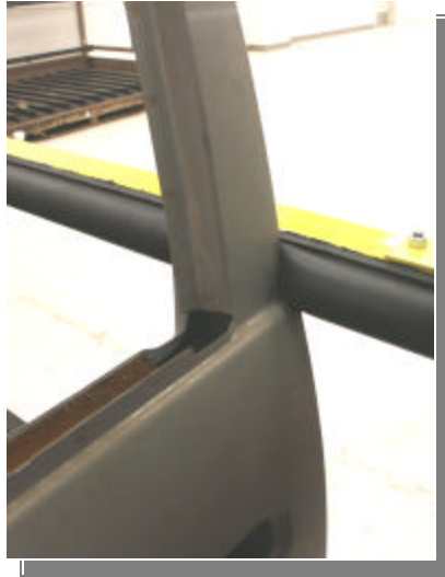
Figure C: Current reconfigurable racking ideas as demonstrated by DaimlerChrysler (prototypes, not yet used in production) – This design features a form fitting “Gumby dunnage” which temporarily molds to the shape of the part contained by the rack.
