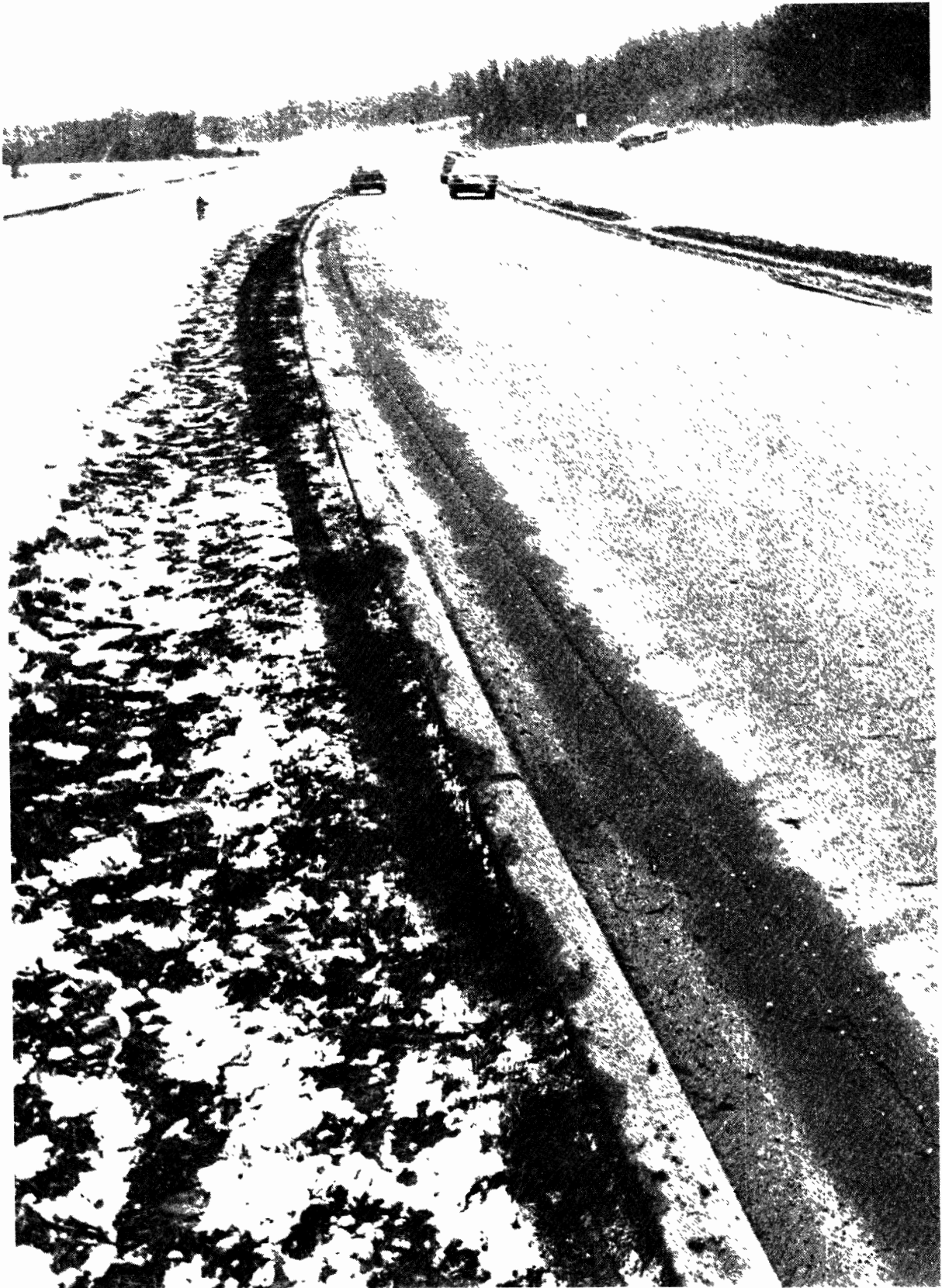
Figure 9.2-2. Path of Pinto that left roadway of urban parkway. Vehicle is in final resting position on right upslope of bank. (AA 344).
