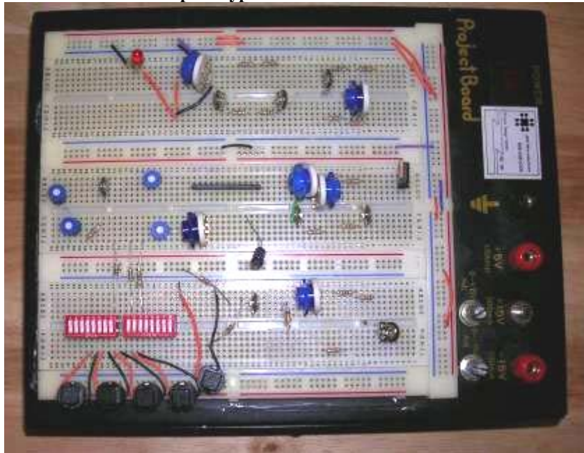
Figure 19: An electronic projected board such as this may used to build a control circuit for the prototype
