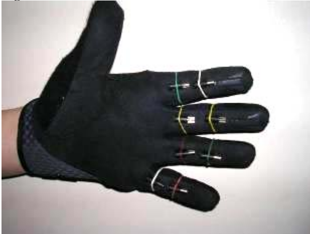
Figure 16: Motors with an eccentric mass will be attached to the glove in the locations shown
