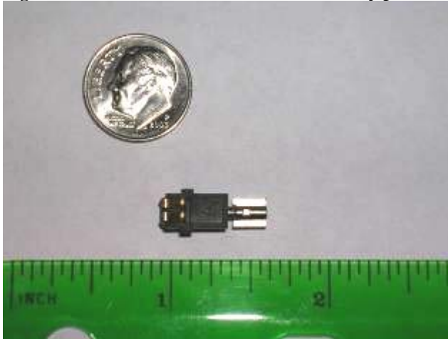
Figure 18: Small size of motors allows for easy placement on the glove, flexibility, and comfort for the user
