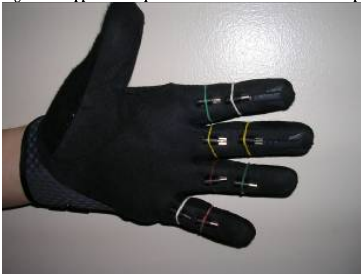
Figure 29: Approximate placement of motors shown on concept prototype
