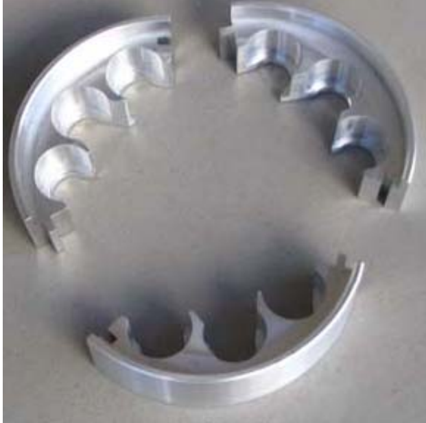
Fig 3. The piston-con-rod alignment tool designed by a previous ME 450 group [2]
