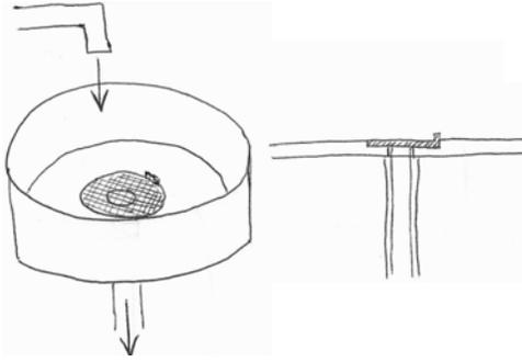
**Open Coarse Screen Filter** Another idea was a coarse screen filter that is open to the atmosphere. The fluid enters a tank and flows out through a screened drain in the bottom. The screen has either a tab or a handle attached for easy removal and cleaning. This design would violate our objective of enclosing all system components for safety and cleanliness. A picture of the concept from the top and also directly from the side are shown to the right.
