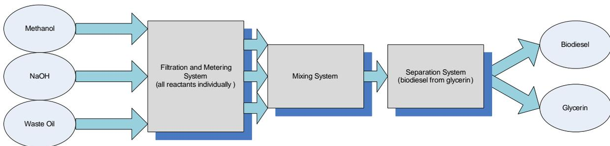
**Figure 2. General waste cooking oil conversion process**
