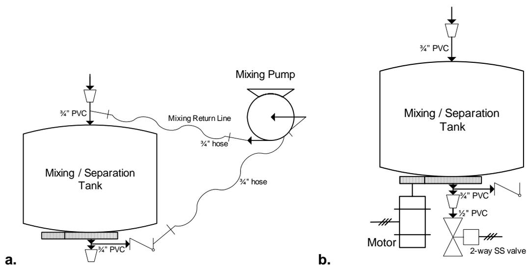
**Figure 22. (a) Mixing pump setup and (b) Separation setup**
