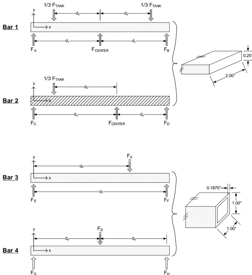
**Figure 13. Support beam free body diagrams**
