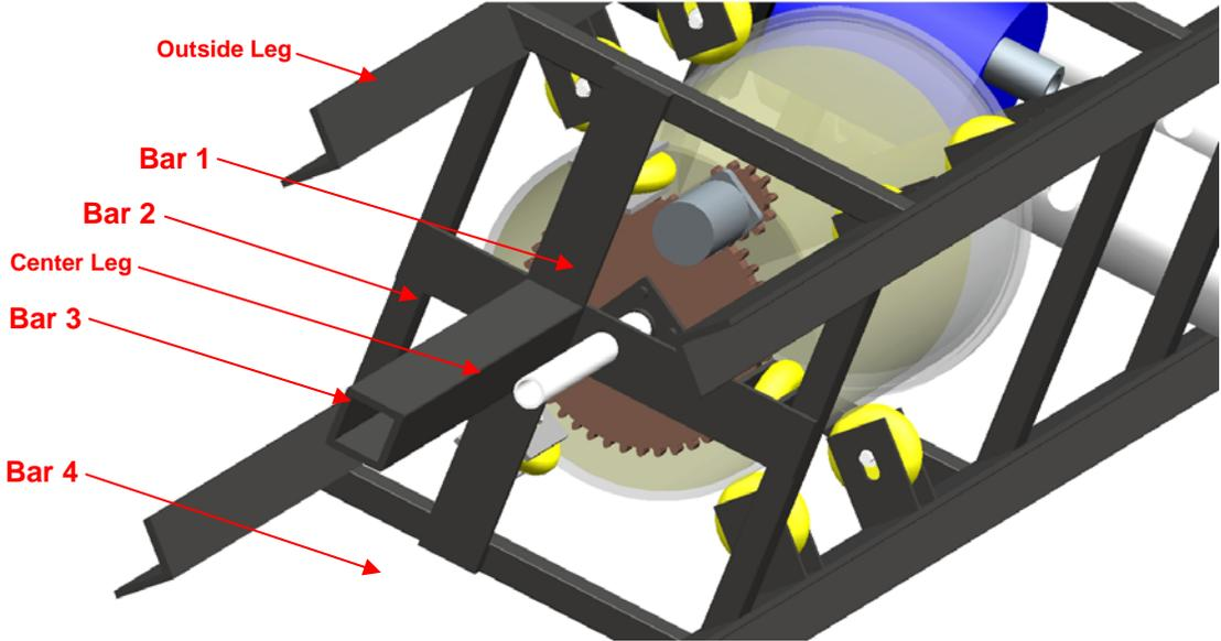
Figure 12. Tank support structure
