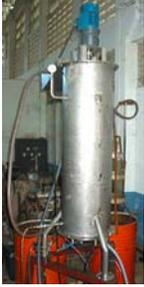
The Deepthort 100B, designed by a Professor in Thailand, was produced for less than \$2,000. It is capable of batch sizes up to about 26 gallons. Since palm-oil is abundant in Thailand, the system was designed to use this it as the feedstock. It is capable of performing other tasks besides basic biodiesel production, such as pre-washing the oil, drying the oil, and recovering methanol.
