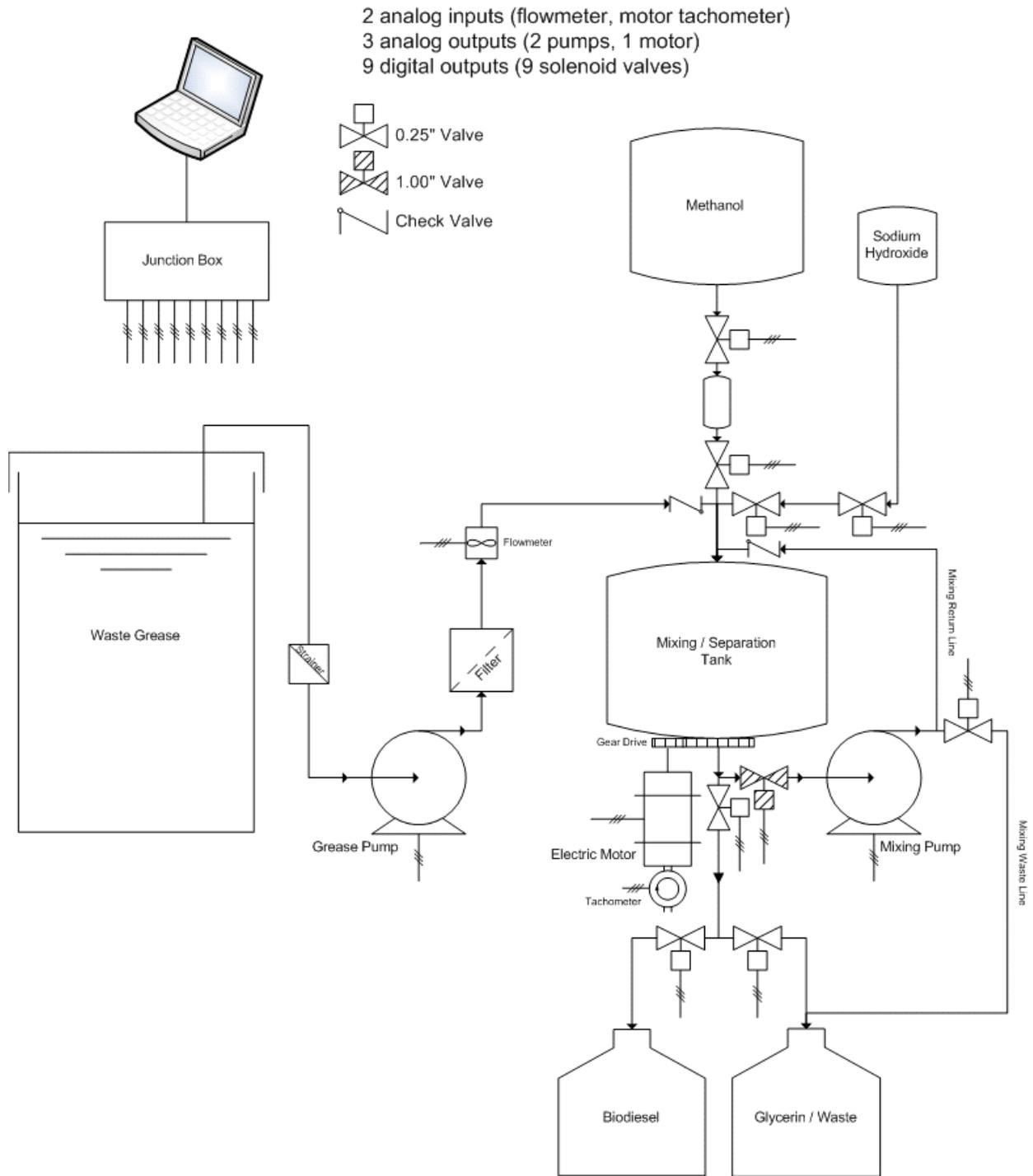
Figure 6. Waste cooking oil conversion system schematic diagram
