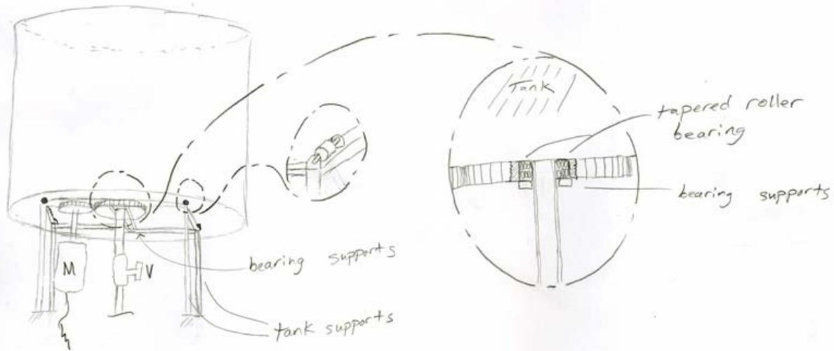
**Figure 5. Detailed view of main separation tank support and bearing system**
