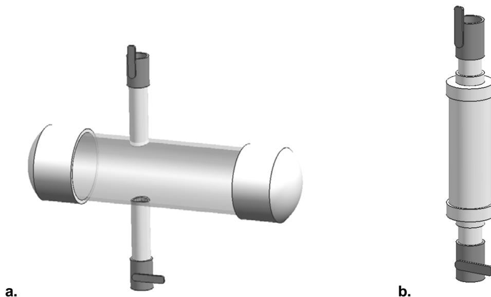
**Figure 21. (a) Methanol intermediate metering tank and (b) NaOH metering pipe**
