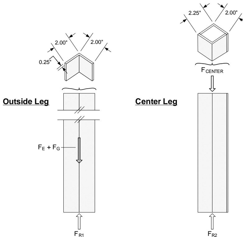
**Figure 14. Vertical beams for support structure**
