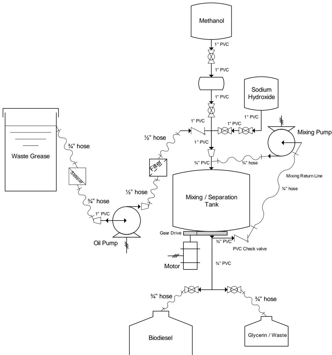
**Figure 19. Final prototype design schematic**
