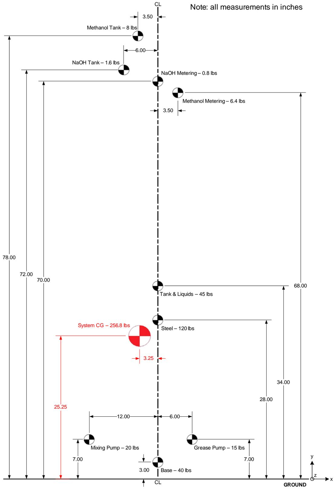
Figure 16: Center of masses for individual components and final COM for system
