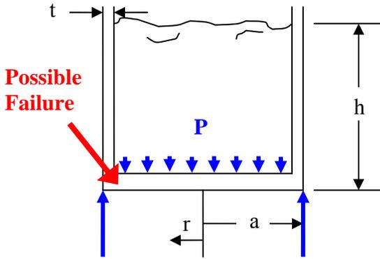
**Figure 15. Free body diagram of the tank supporting 40 lbs. of fluid.**
