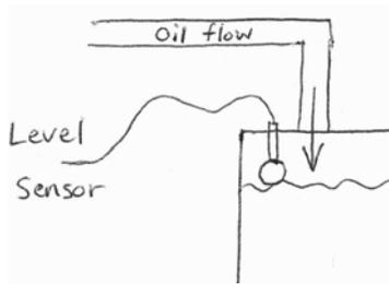
**Oil Pumped to Set Level** This concept uses the gravity feed process for the methanol and sodium hydroxide assuming that the system height is still reasonable with these tanks. After opening the valves for these tanks, the oil would then be pumped into the mixing tank until the total fluid level achieves the correct volume of oil measured by when it reaches the correct height in the tank. A level sensor would provide the feedback to the control unit to
