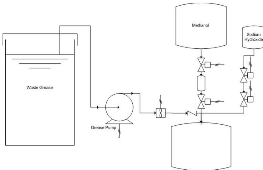
**Figure 4. Reactant input concept selection (not showing other components)**
