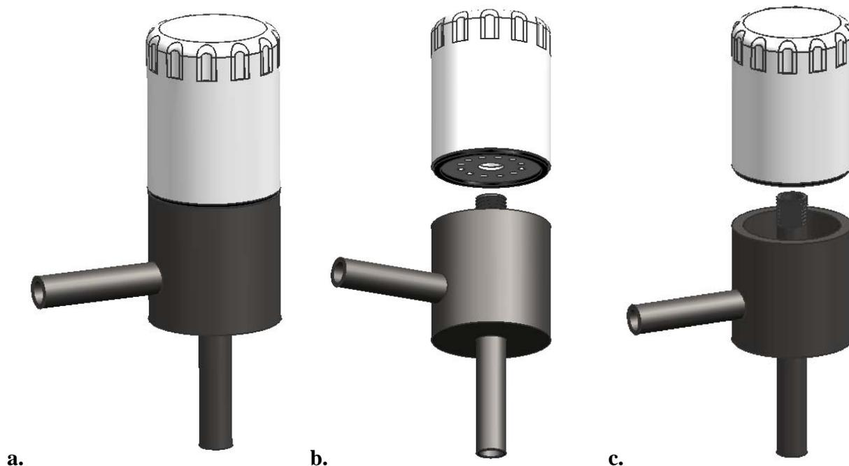
**Figure 20. Oil filter with coupling (a) connected together (b,c) exploded to show connection**
