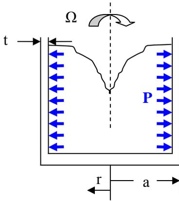
**Figure 16: Free body diagram of the tank walls retaining rotating fluid.**
