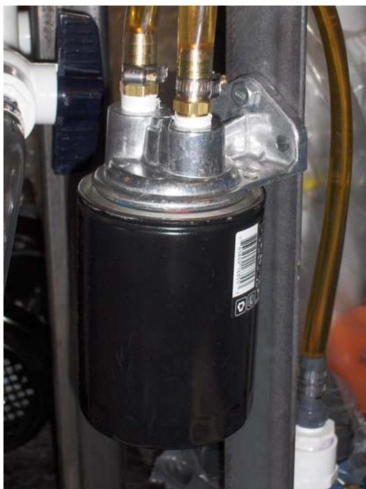
**Figure 26. Cartridge filter used in prototype.**
