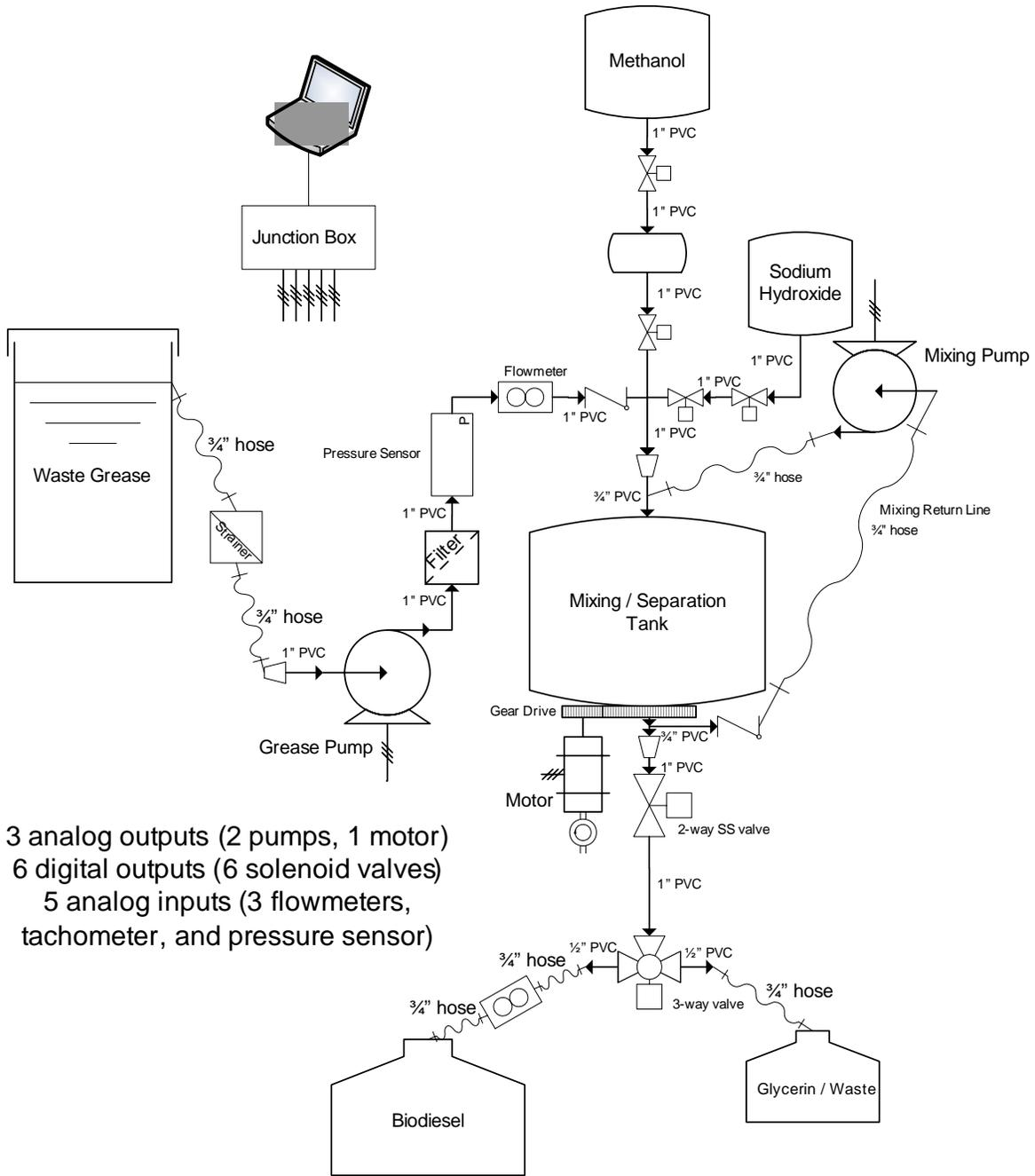
Figure 25. Final full-scale design schematic
