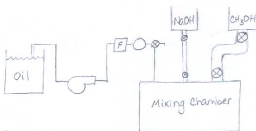
**Oil Pumped through Flow Meter** A flow meter located in the oil line can be used to determine the velocity of the fluid. The velocity of the fluid multiplied by the cross-sectional area of the pipe results in the volume flow rate. By performing a time integration of the volume flow rate in our control software, we will shut the pump off when one batch's worth of oil enters the tank. This
