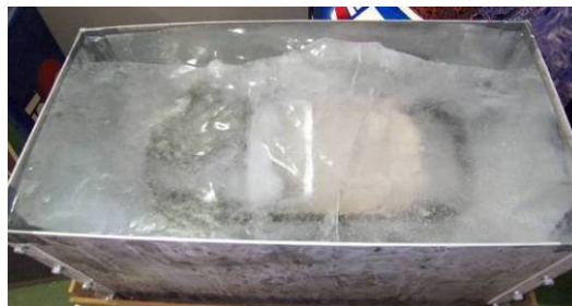
Figure 33: Prototype after interval freezing (top view).
