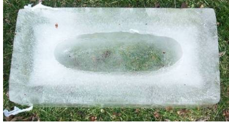
Figure 31: Hollow center of prototype ice.
