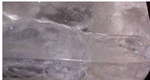
Figure 32: The ice crack occurred during the freezing.
