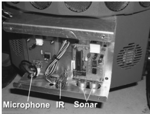
Figure 3. Three sensor modalities were mounted in front of the robot, pointing downward: A microphone, an infrared range sensor, and an ultrasonic range sensor.
