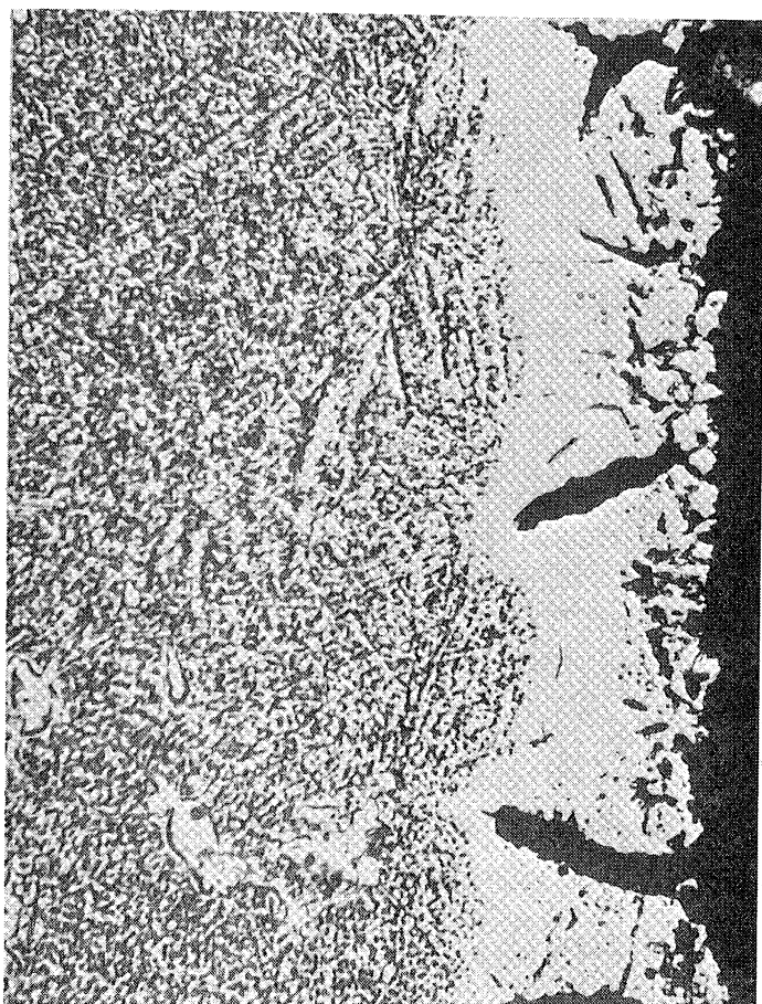
Figure 31 Specimen R-12 (Longitudinal Section to Show Surface Attack) Exposed Without Stress 10 Hours at 1800°F
