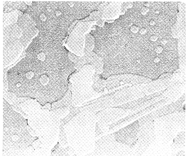
Figure 48 8200x Specimen R-45 Creep-Exposure 100 Hours at 1800°F to 5.17% Deformation
