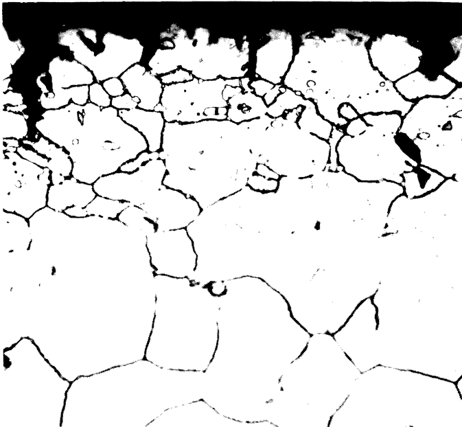
Figure 59 Spec. No. R-99 (Section Showing Surface Attack) Creep-Exposure at 1300°F for 100 Hours to 0.63 Percent Deformation
