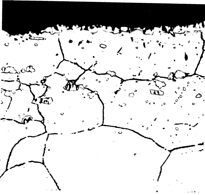
Figure 61 Spec. No. R-93 (Section Showing Surface Attack) Exposed Without Stress 100 Hours at 1400°F
