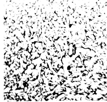
Fig. 42. Ti 150A 1350°F Water Quench + 16.7 hrs at 1000°F and 15,000 psi - X1000D
