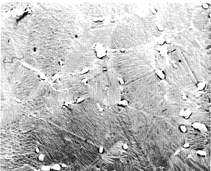
Figure 14. Chromel-AS 1550°F --four hour + Air Cool
