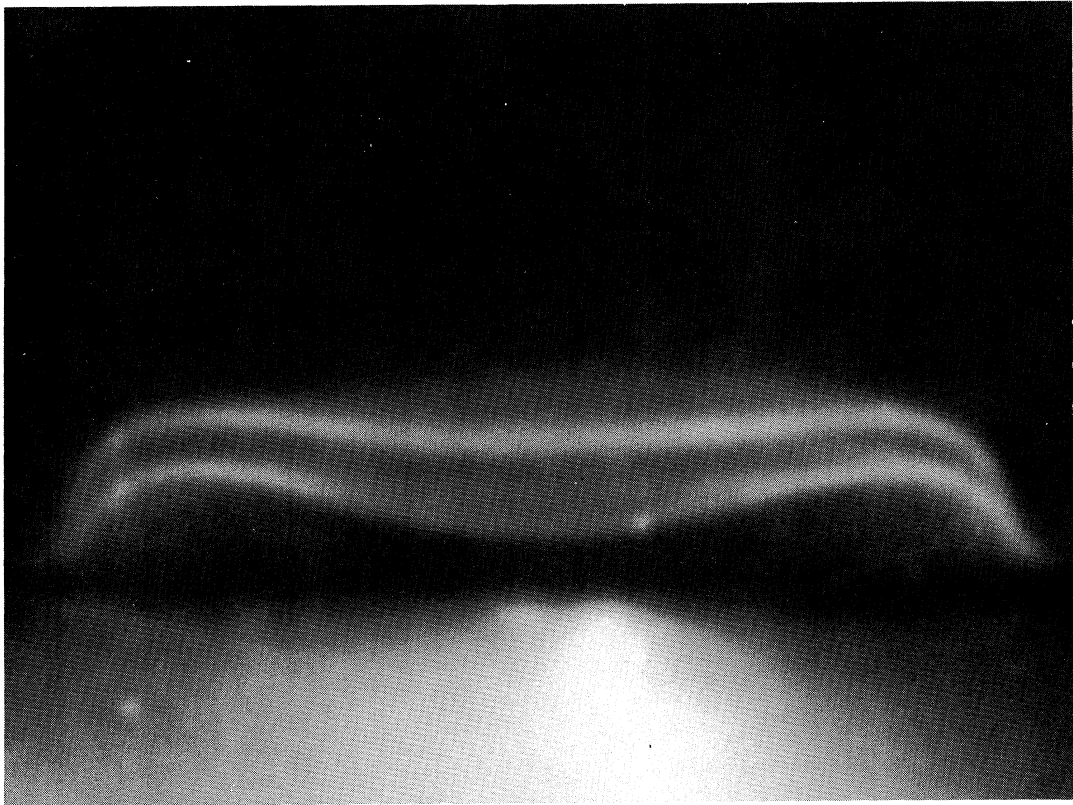
Figure 3. Ethane flame - ozone present in lower flame
