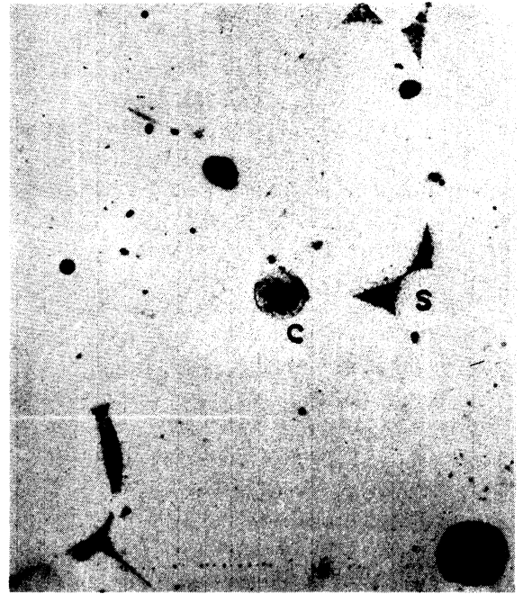
(c) Autoradiograph 250X (4-day exp.) annealed 15 hours at 1200°C, water quench.
