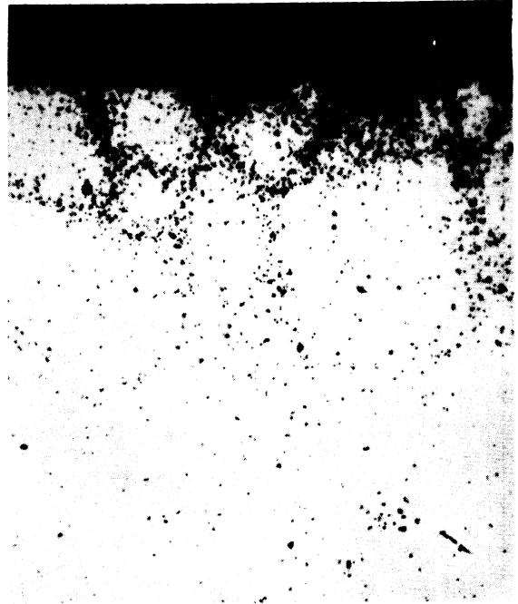
(b) Diffused 220 hours at 1300°F Autoradiograph of unetched metal surface
