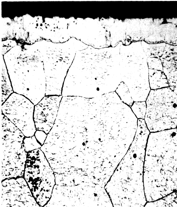
(c) Diffused 220 hours at 1300°F Photomicrograph of etched metal surface
