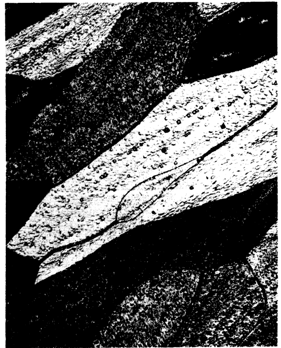
(d) Same field as (b) after deep etching with 20% ammonium persulfate to show sub-grain structure. Photomicrograph 75X
