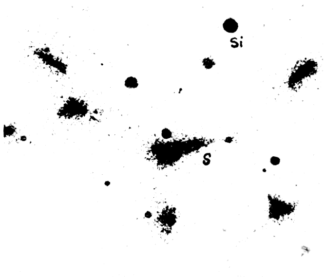
Fig. 14 Sulphide Identification in Fe-Si-S Alloy. Iron with 0.50% silicon and 0.20% sulphur (low activity), annealed 15 hrs. at 1200°C, water quench. Autoradiograph 500X (10-day exp.)
