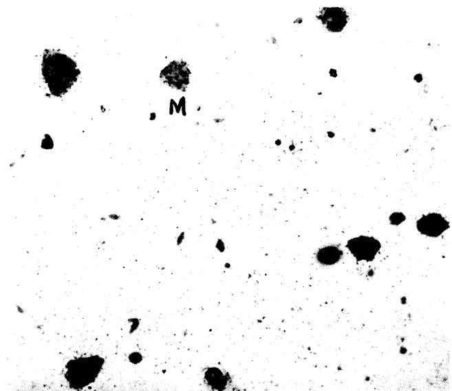
Fig. 15 Effect of Manganese on the Sulphide Microstructure. Iron with 0.50% manganese and 0.20% sulphur (low activity), annealed 50 hrs. at 950°C, water quench. Autoradiograph 500X (4-day exp.)
