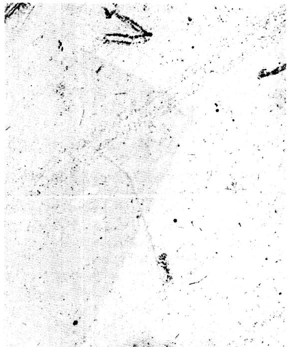
(d) Second autoradiograph over same field as (c) and exposed for 14 succeeding days.
