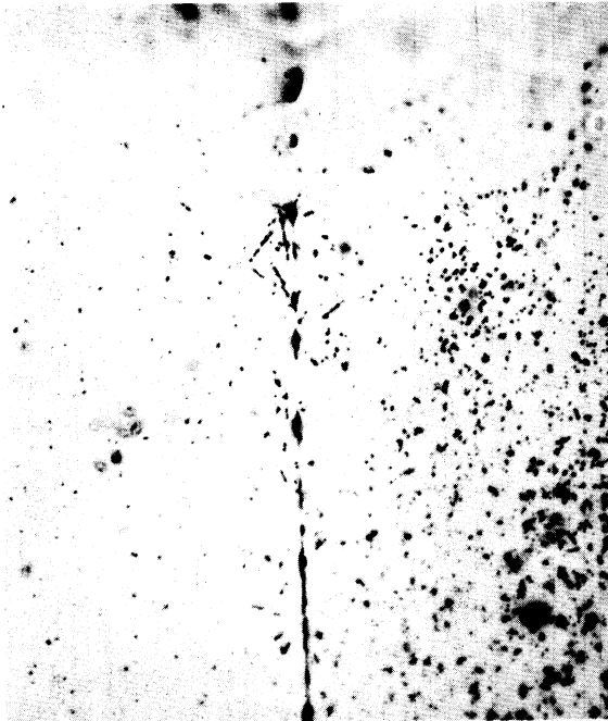
(b) Grain Boundary Showing Autoradiographic Evidence for Presence of Polonium Autorad. Expos. Time: 14 days
