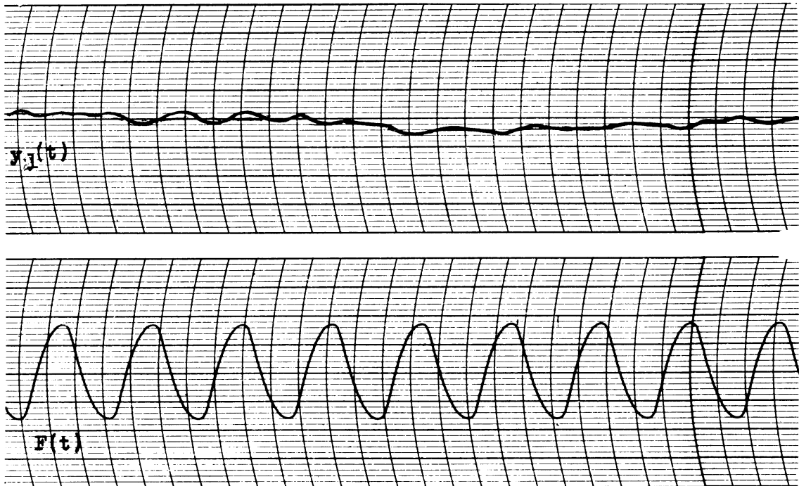
Figure 4-12. Response y_1 amplified 50 times more than F(t) .
