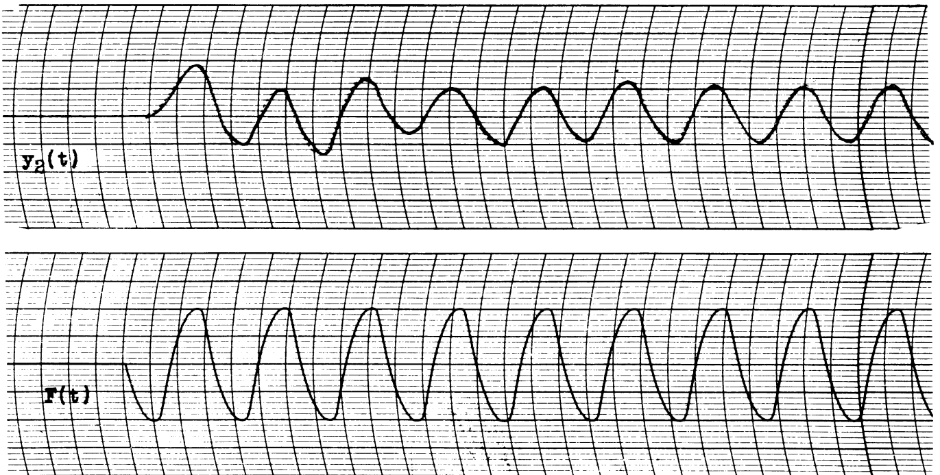
Figure 4-13. Response y_2 and driving voltage F(t) (with equal gains) for a dynamic vibration absorber.
