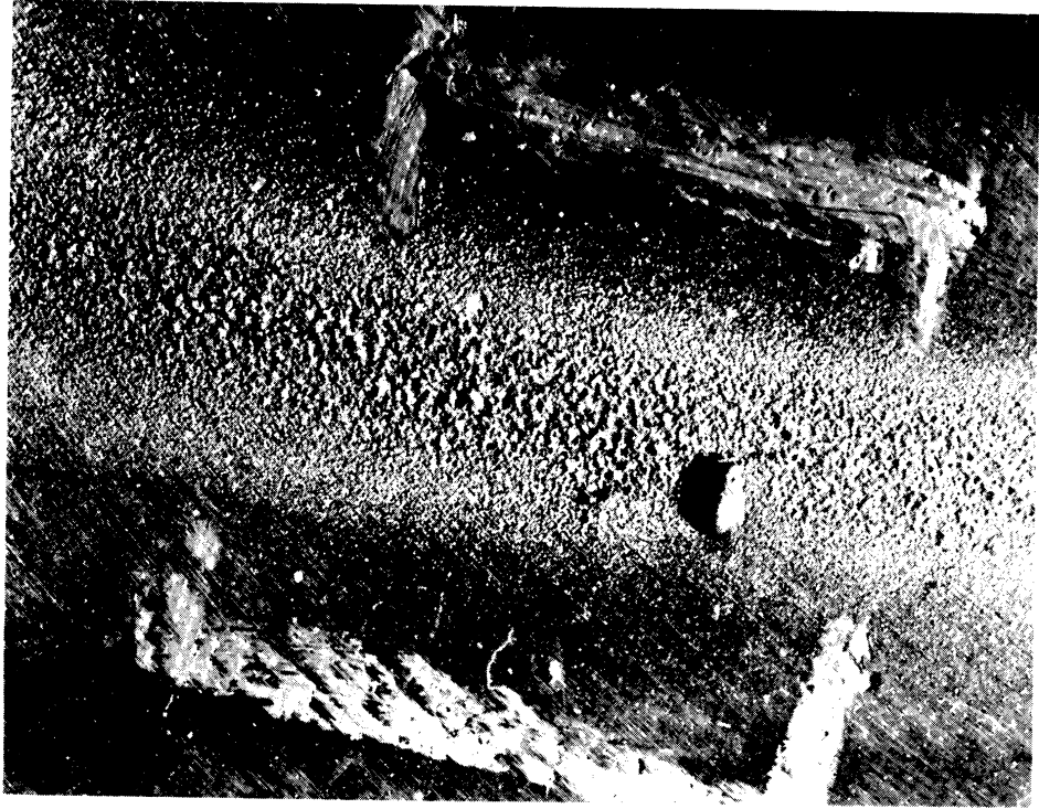
Fig. 12 Cavitation Erosion - Mercury Pump
