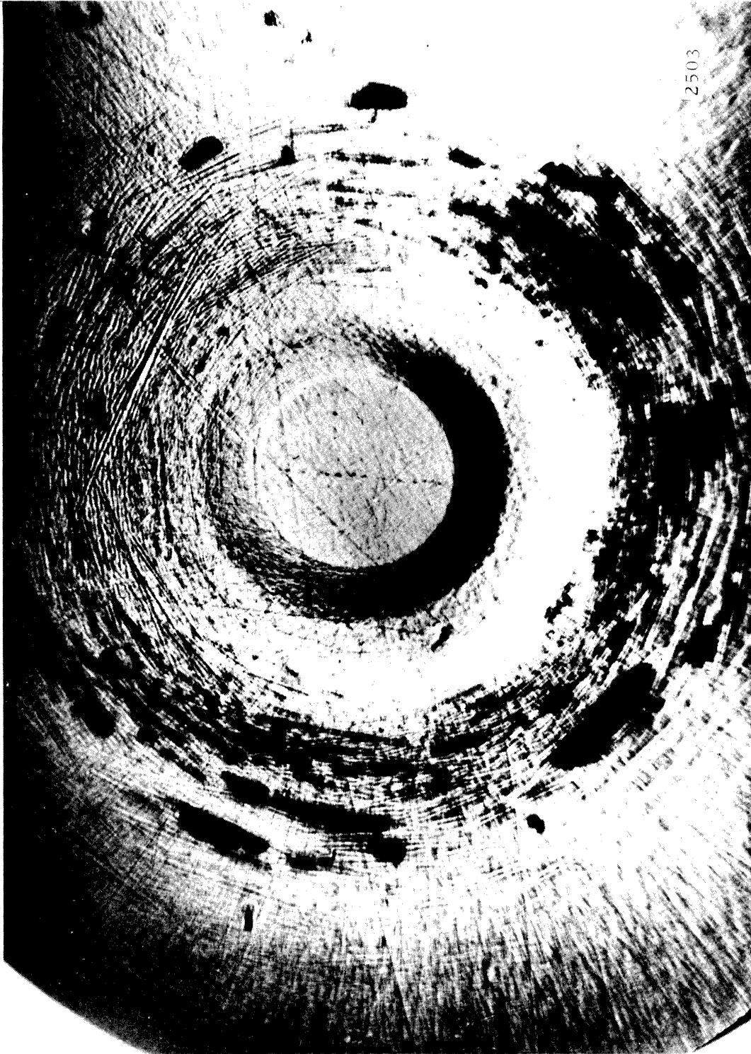
Figure 4. Water Droplet Impact Crater on Plexiglas, Magnification 100 x. (After A. Fyall, RAE, Farnborough, England).
