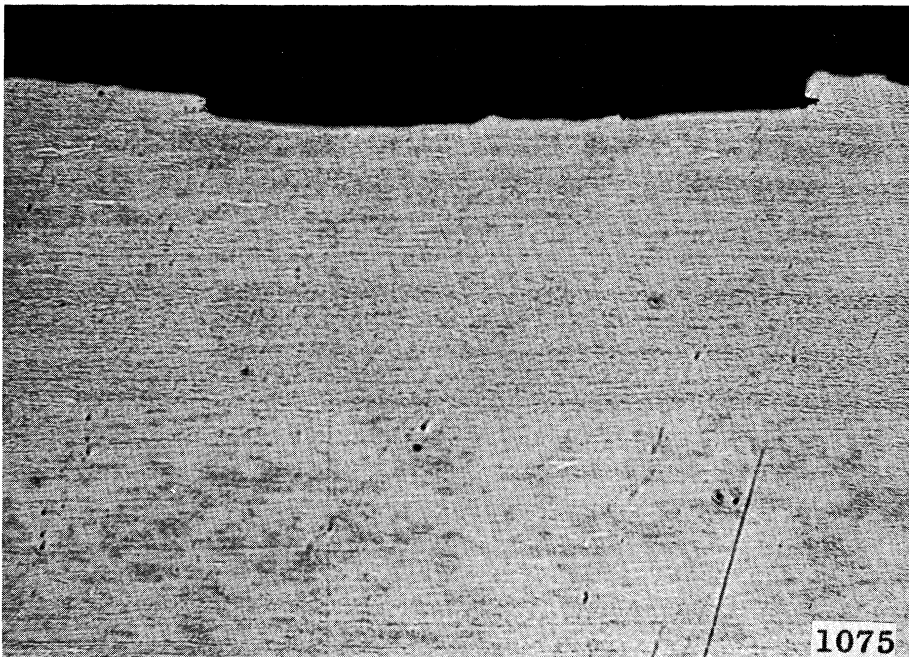
Figure 21. Microsection Through Gross Damage Area on Numbered Side of Sample Number Cb-1Zr 20 as Shown in Figure 58. Etched. Magnification 100X.
