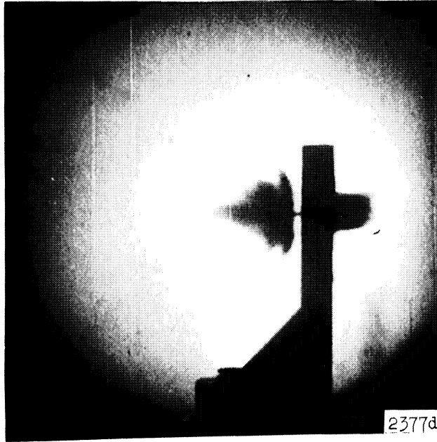
Fig. 3. - Liquid jet from momentum exchange device showing the standing wave type of instability observed in some cases.
