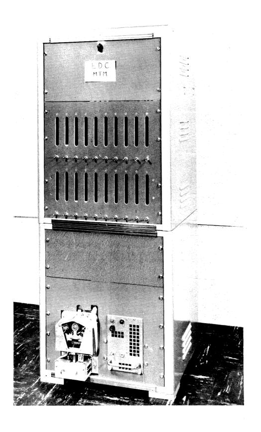
Figure 1. The Electronic Data Collector Showing the Counters, Tape Punch and Power Supply.
