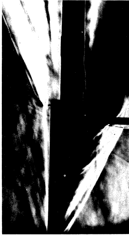
(g) p_{0j} = 101.8 \text{ psia} , w^* = .0005'' , p_{0j}w^*/p_{\infty}L = .091 Laminar separation
