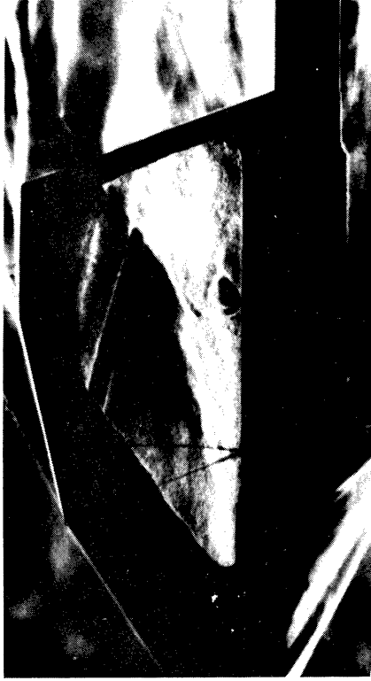
(f) p_{0j} = 69.2 \text{ psia} , w^* = .0031'' , p_{0j}w^*/p_{\infty}L = .369 Turbulent separation
