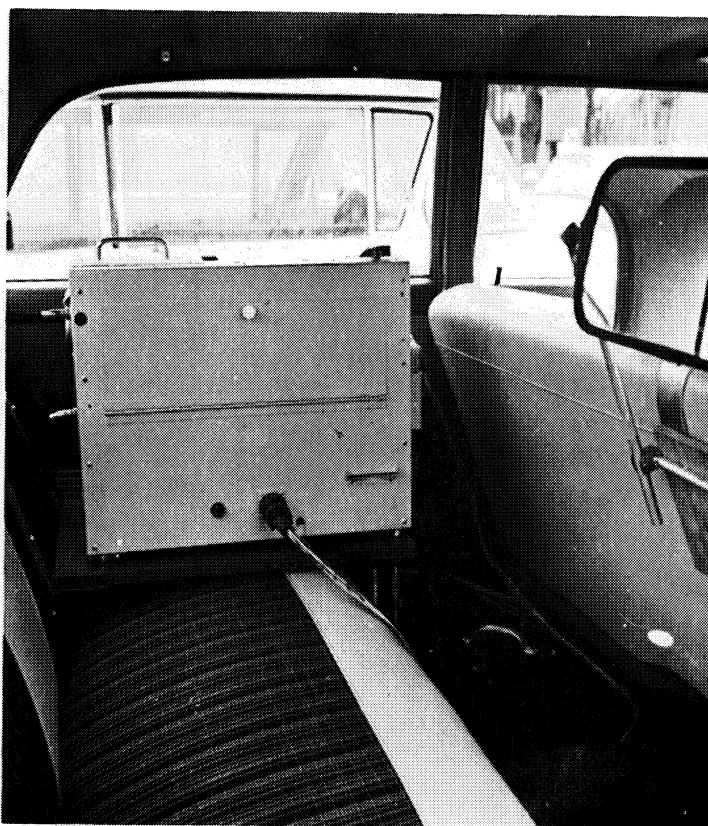
Figure 8. Photograph of Interior of Test Car Showing Data Box Mounted on Rear Seat. Mirror Mounted on Rear of Front Seat Provides Reflected Image of Highway Behind Test Car for Camera Mounted on Deck Behind Rear Seat.
