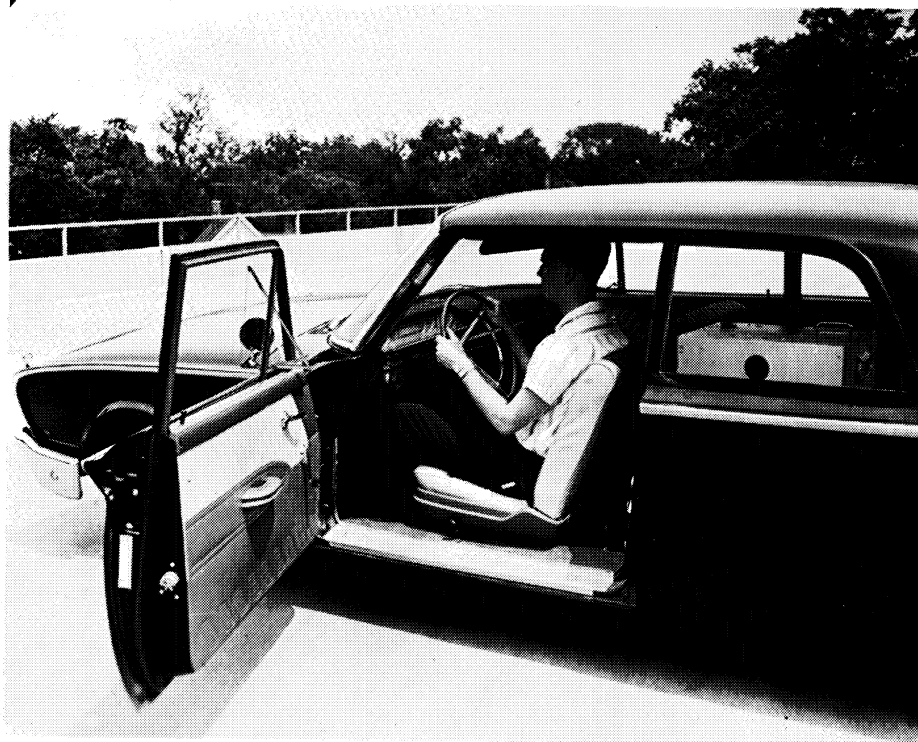
Figure 7. Photograph of Driveometer Installed in Test Car Showing Data Box on Back Seat Directly Behind the Driver.
