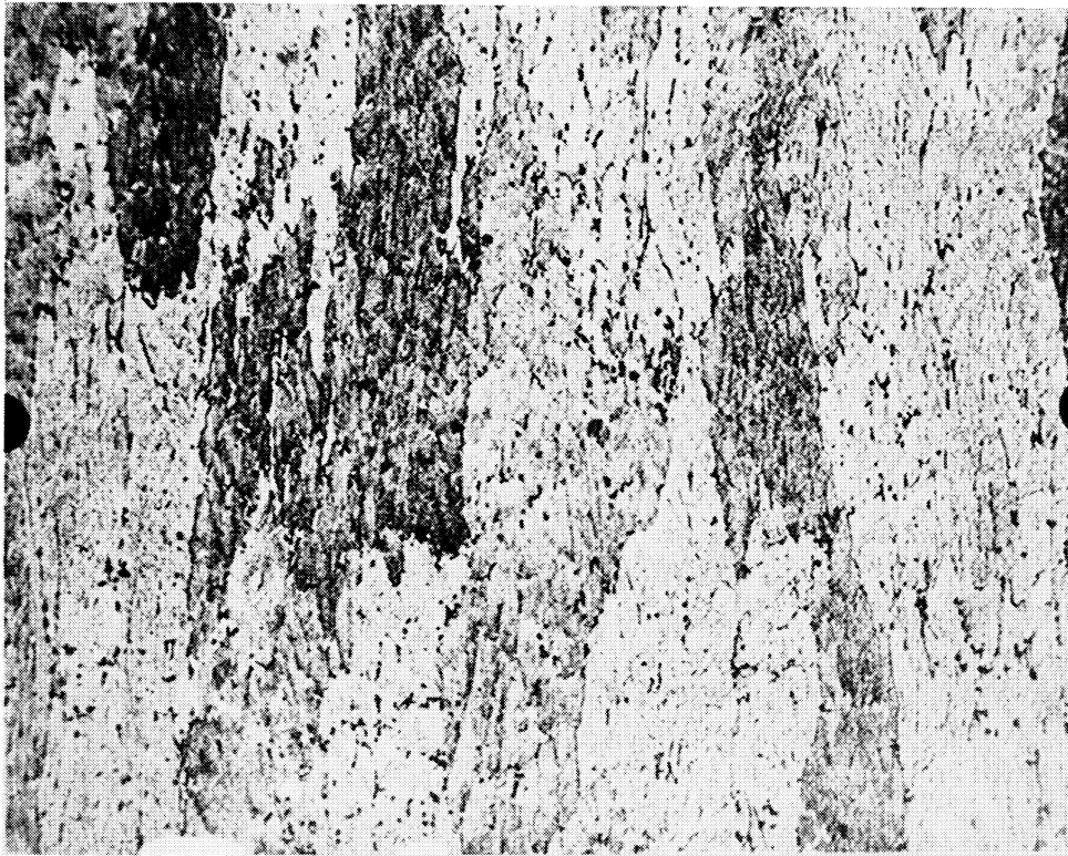
Figure 15. 2024-T4 Aluminum, Solution Heat Treated (100 X, Keller's Etch).
