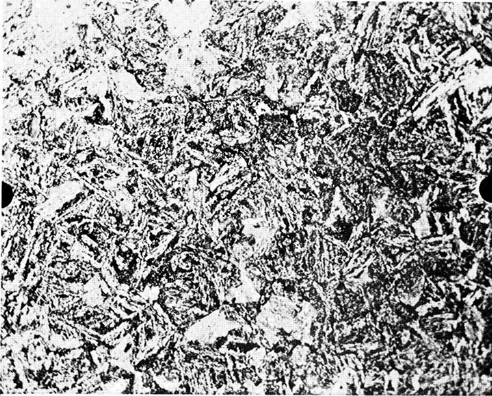
Figure 13. AISI 4340 Steel, Hot Rolled (100 X, Nital Etch).
