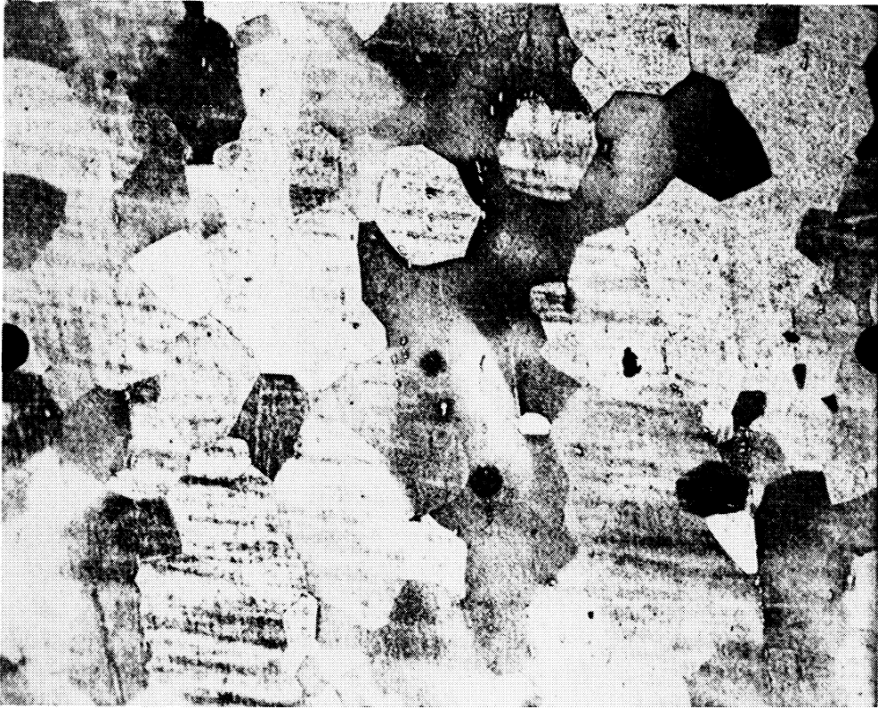
Figure 17. Molybdenum, Arc Cast and Extruded (100 X, 50% HNO 3 Etch).
