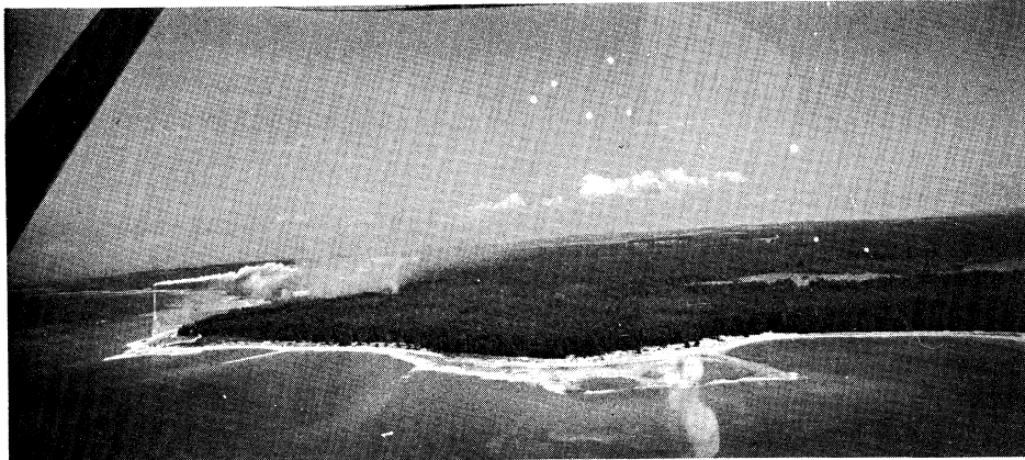
Fig. 15. Side view of plume traveling over land. Picture shows little diffusion close to source but a rapid breaking up of the plume as it encounters mechanical turbulence caused by wind traveling over rough land surface.
