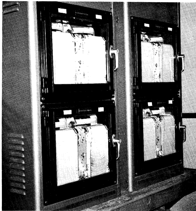
Fig. 8. Wind speed and wind direction recording panel. Four dual channel Esterline Angus recorders record wind speed and direction at each of four levels, 32, 64, 128, and 256 ft above lake level.
