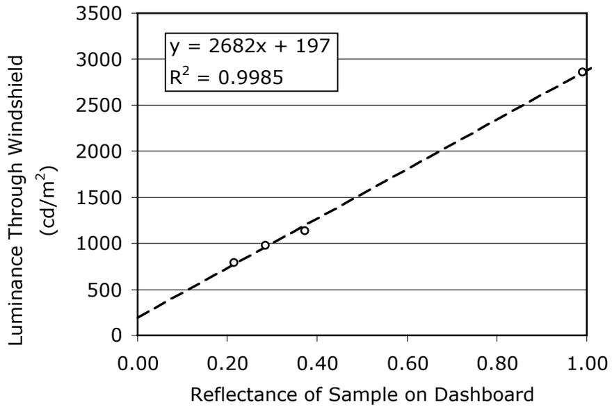
Figure 3. An example of the regression modeling used to separate luminance attributable to dashboard reflection and residual scatter, for a single vehicle. The luminance at the vertical-axis intercept (in this case, 197 cd/m<sup>2</sup>) is the estimate of “residual scatter” luminance.
