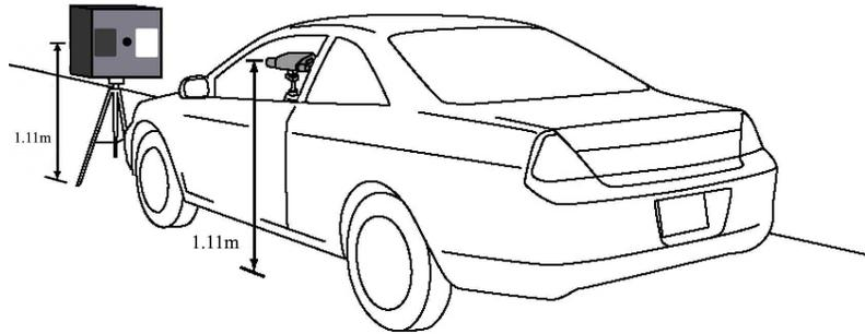
Figure 1. Diagram of the experimental setup. The heights of the spectrophotometer and light trap shown here (1.11 m) were used for passenger cars. The black dot on the box in front of the car represents the opening of the light trap.
