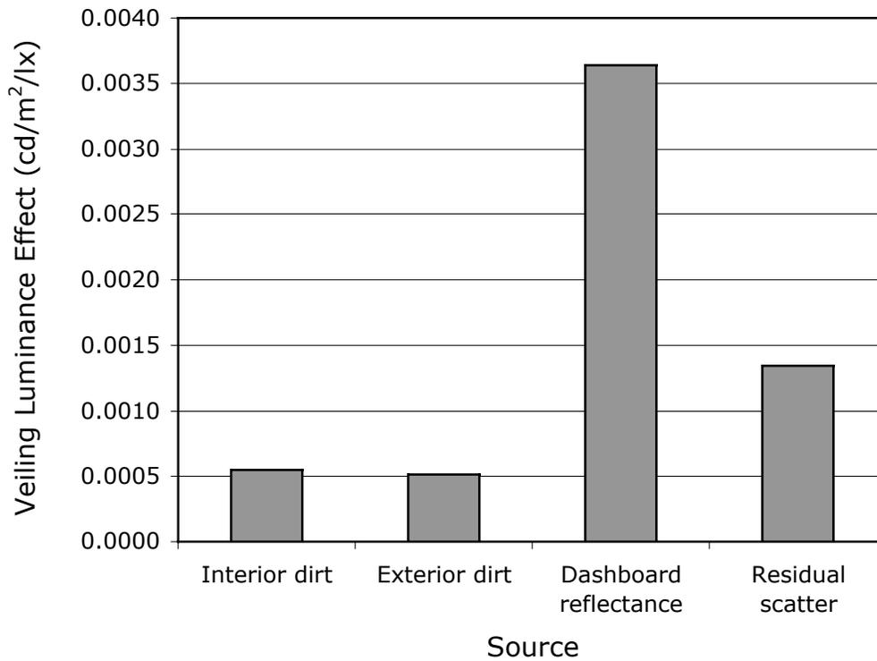
Figure 4. Mean luminance effects (cd/m<sup>2</sup>/lux) for the sources of veiling luminance.
