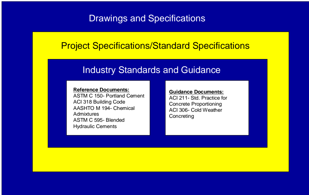
Figure 1. Concrete Specifications Terminology Hierarchy
