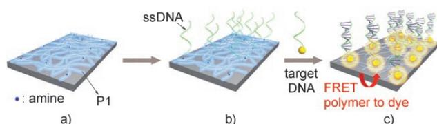
**Figure 1.** Schematic representation of the signal-amplifying conjugated polymer-based DNA chip. a) **P1**-coated glass slide by covalent bonding; b) light-directed on-chip oligonucleotide synthesis; c) hybridization with a target DNA results in large emission enhancement of the fluorescent dye through efficient Förster resonance energy transfer.
