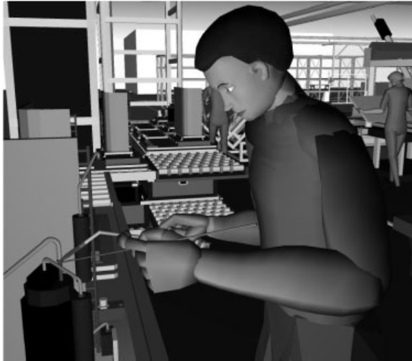
Figure 1 A typical digital human figure model for static reach, fit, and line-of-sight analysis using Jack software (courtesy of Ulrich Raschke, UGS-PLM Solutions, Ann Arbor, Michigan, USA).
