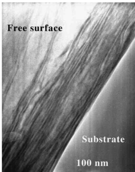
Figure 10. Cross-section image of the (\{Ag_{66}E6\}/PSS)_{24} multilayer deposited on a polystyrene substrate by TEM. Dark lines correspond to the silver domains localized in the nanocomposite layers. The top of the structure has been slightly damaged probably during microtoming.
