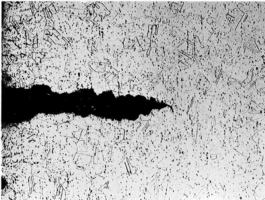
Fig. 24. Thermal Crack in Type 304 Stainless Steel 100X
