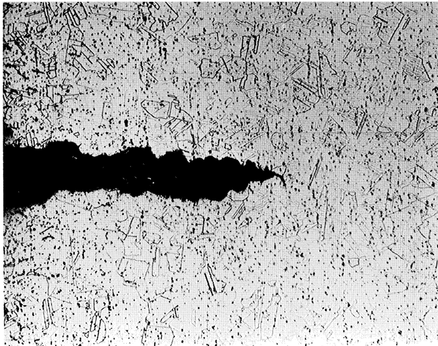
Fig. 25b. Thermal Crack in Type 304 Stainless Steel. X100
