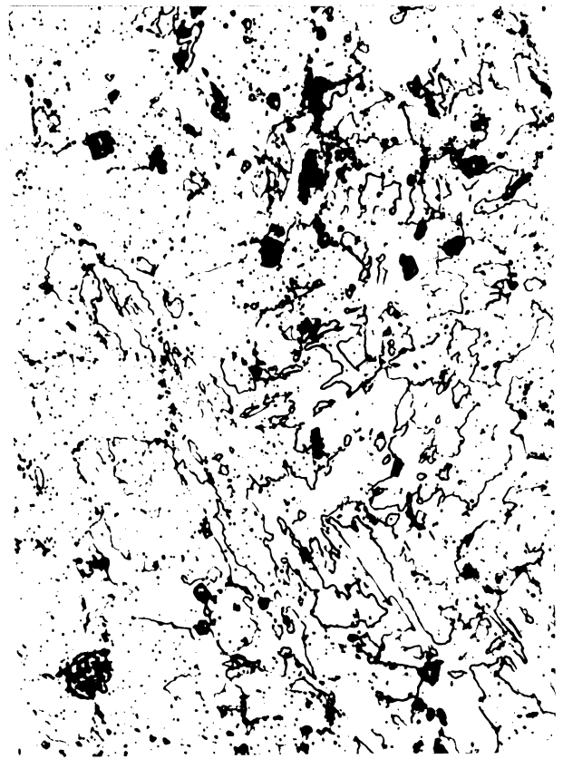
B. Normalized 1950°F, tempered for 6 hours at 1250°F to 293/311 BHN.
