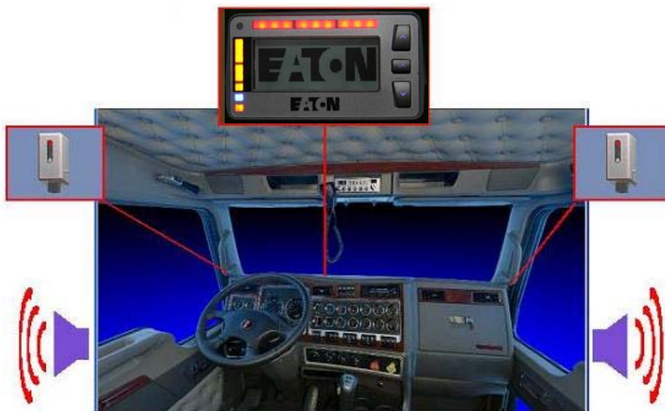
Figure 39. Heavy-truck DVI space in truck cockpit
