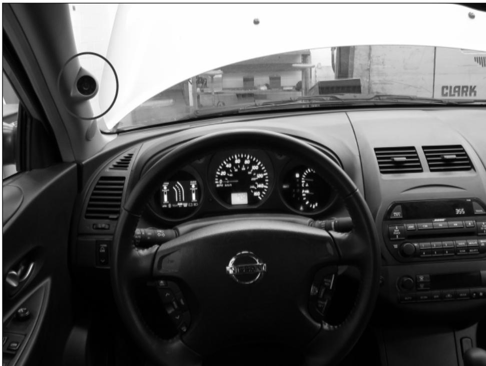
Figure 2. Inside an RDCW FOT vehicle. One camera was retrofitted to the A-pillar (circled in the figure).
