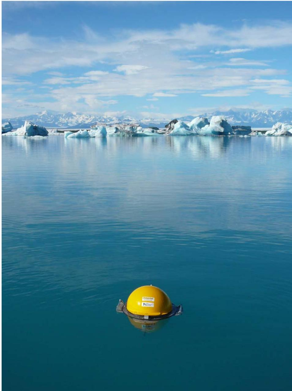
**Figure 3. ALWAS is an autonomous drifter buoy that measures various water quality parameters, including turbidity, as a function of location. ALWAS was deployed in Vitus Lake during the 2006 and 2007 summer field seasons.**
