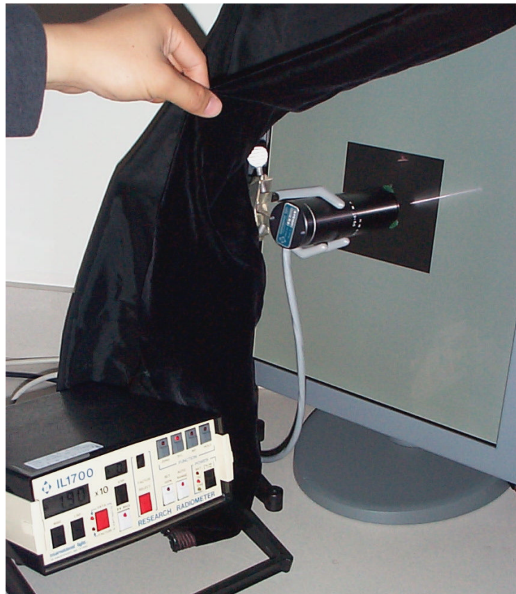
Figure 3.5: Luminance measurements setup with IL1700.
