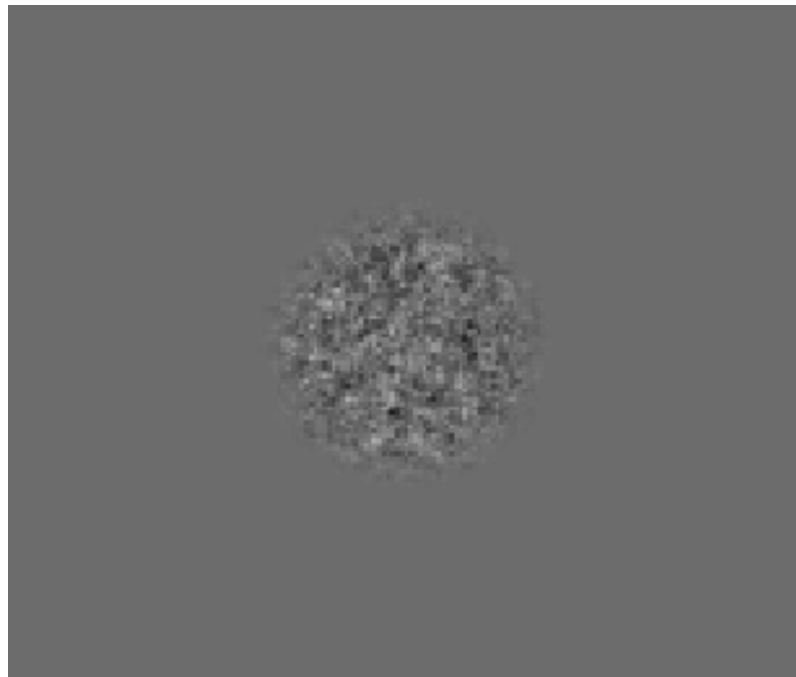
Figure 6.6: Close-up image of a filtered noise pattern used in the 2AFC contrast threshold test. The actual target size was 145mm in diameter. The pattern simulates quantum mottle in an indirect digital radiography system.
