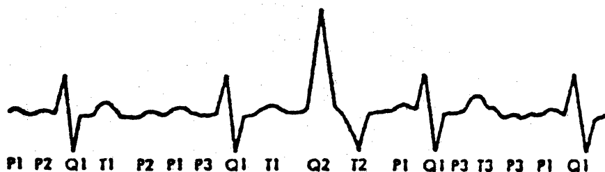
Fig. 4. Passage of an electrocardiogram that has been coded for arrhythmia analysis. Each QRS type is designated Q1, Q2, and so on where Q1 represents the dominant beat and Q2 an ectopic beat. P and T waves of different morphologies are similarly coded. This example shows atrial fibrillation with a ventricular ectopic beat. (Reproduced by permission from Computers and Biomedical Research . 24 )
