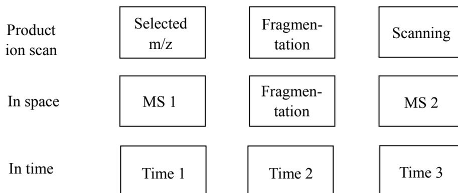
Scheme 1-1. Comparison of a product ion scan by space-based and time-based tandem mass spectrometers. The scheme is adopted from reference [28].
