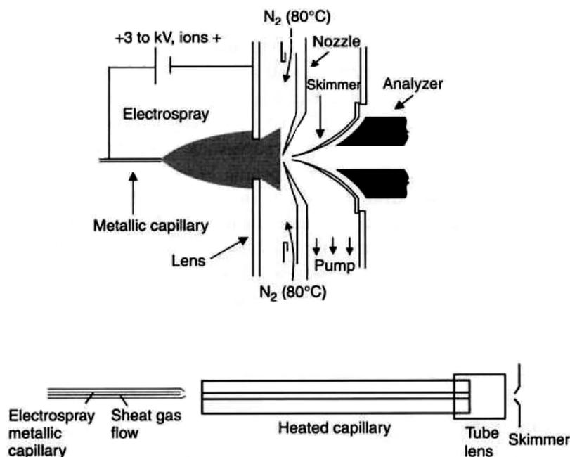
Figure 1-2. Diagram of ESI source with a curtain of heated nitrogen to assist desolvation (top), or with a heated capillary for desolvation (bottom). This figure is reproduced from reference [28] with permission.
