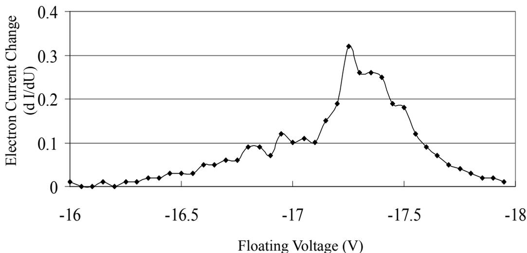
Figure 3-4. Electron energy distribution at an applied cathode bias voltage of - 18.0 V and extraction lens voltage of - 19.0 V. The heating current was 1.8 A.
