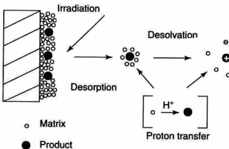
Figure 1-3. Diagram of the principle of MALDI. This figure is reproduced from reference [28] with permission.
