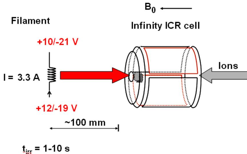
Figure 2-2. Schematic diagram of a directly heated filament EDD configuration.
