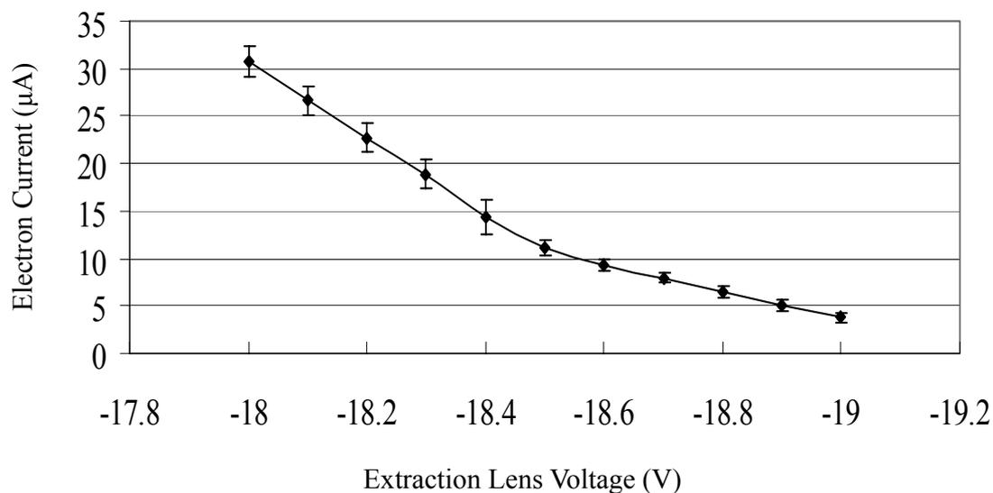
Figure 3-3. Electron current through the ICR cell as a function of extraction lens voltage at fixed cathode bias voltage (- 18.0 V).
