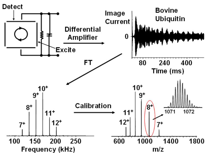
Figure 1-4. Time domain signal from bovine ubiquitin, a 9 kDa protein (upper right) obtained by excitation and detection of ions in an ICR cell (upper left). Frequency domain (lower left) FT-ICR signal is obtained through Fourier transformation and the corresponding mass spectrum (lower right for multiply charged bovine ubiquitin) is obtained by applying the equation  $\omega = zeB/m$ . The inset shows the baseline isotopic resolution that is routinely attained by FT-ICR.
