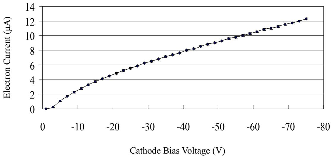
Figure 3-2. Electron current through the ICR cell as a function of cathode bias voltage when the potential difference,  $\Delta U$ , between the cathode and the extraction lens was kept constant (equal to 1 V). The cathode heating current was 1.8 A.
