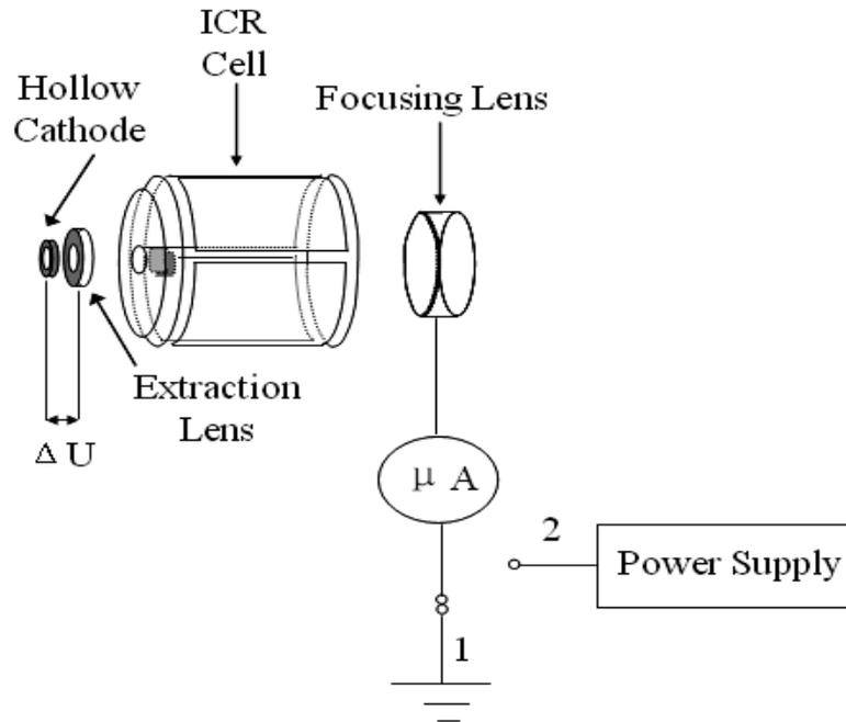
Figure 3-1. Experimental configuration for electron current and energy measurements. The microammeter was connected to ground (1) when measuring electron current through the ICR cell, and connected to a floating power supply (2) when measuring the electron energy distribution.
