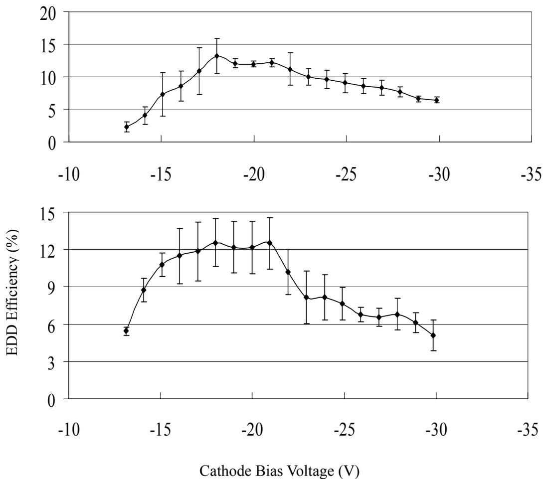
Figure 3-5. EDD efficiency of the oligonucleotide dT<sub>6</sub> (top) and the peptide substance P (bottom) at different cathode bias voltages at fixed electron current ( $\sim 4 \mu\text{A}$ ). The optimum EDD efficiency was obtained at an electron energy of 16-22 eV.
