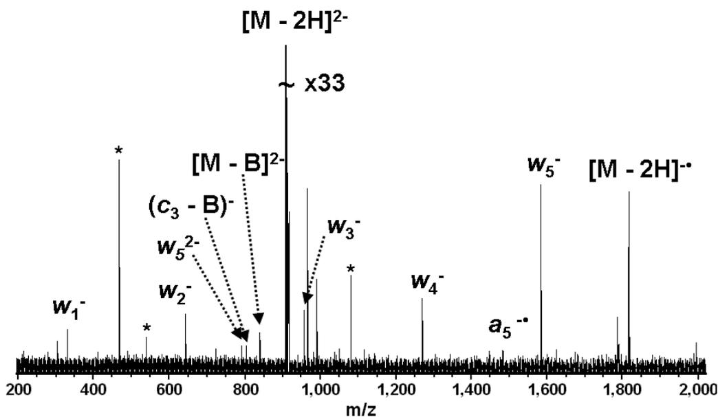
Figure 2-4. EDD (21 eV electrons, 200 ms irradiation, 30 scans) of  $dA_6$  with a heated filament electron source. A complete  $d/w$  (only one label is given) ion series is observed, allowing full sequencing of the oligonucleotide. Electronic noise spikes are labeled with asterisks.
