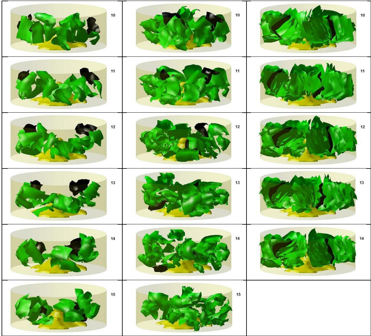
Figure 5.5-14: Illustrative snapshots of the motion of 16 (left column), 32 (middle column), and 64 (right column) cloth pieces with Re = 1.2 \times 10^3 , \Delta t = 5.03 \times 10^{-4} . Snapshots differ by a half agitation cycle, corresponding to the full rotation of the agitator in one direction.
